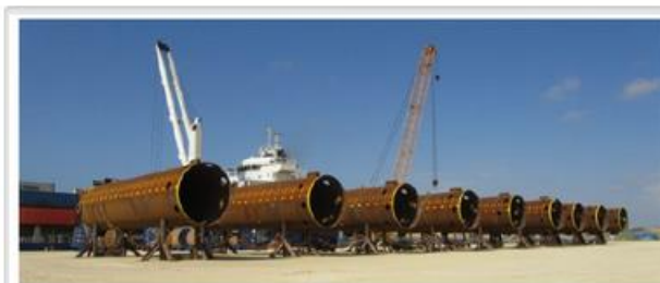
Figure 3: Piles à succons.
