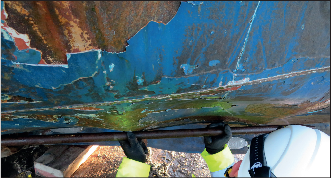
Figure 3: Detail of shell plating damage showing coating loss and indentation between internal frames
