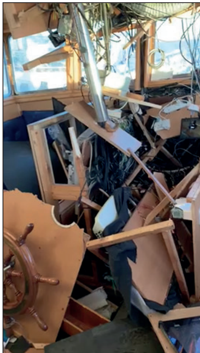
Figure 4: Wheelhouse destruction by shock damage
