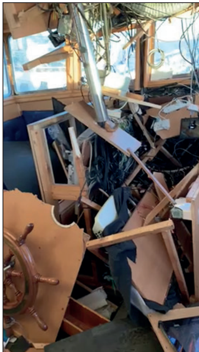
Figure 4: Wheelhouse destruction by shock damage
