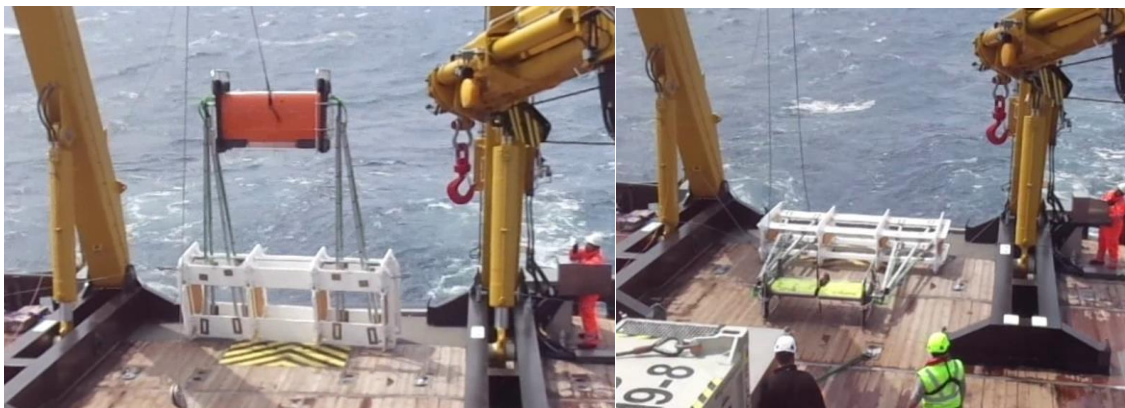
Figure 3-9: ROTV with the fixed frame system for MAG acquisition.
