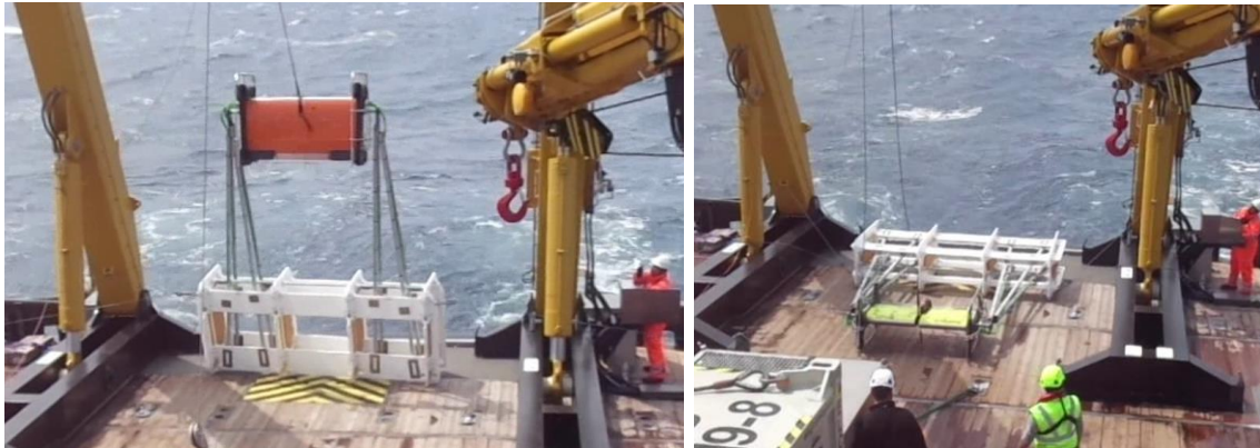
Figure 3-9: ROTV with the fixed frame system for MAG acquisition.
