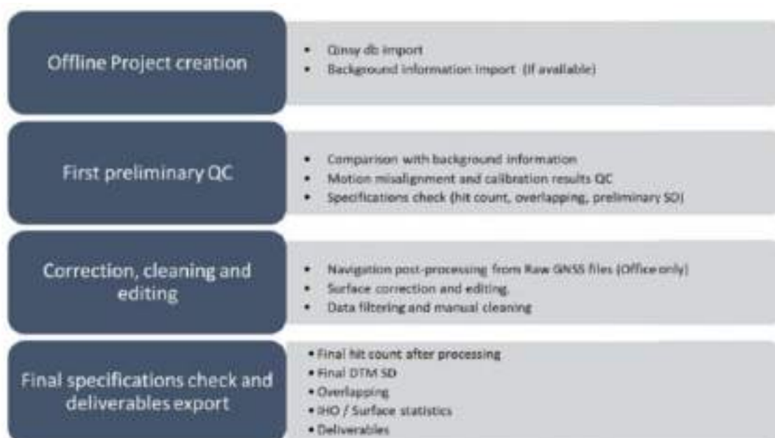
Figure 2-4: MBES bathymetry processing overview.
