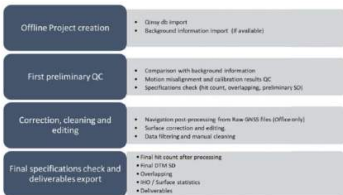
Figure 2-4: MBES bathymetry processing overview.
