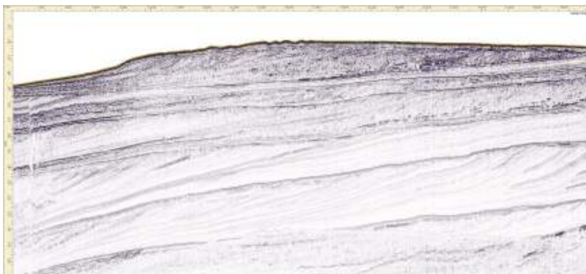
Figure 2-8: Zero-phase corrected control stack (Demultiple, Noise filtering, Deghost, Static Correction, Far Trace Mute & Pre-Stack Migration).
