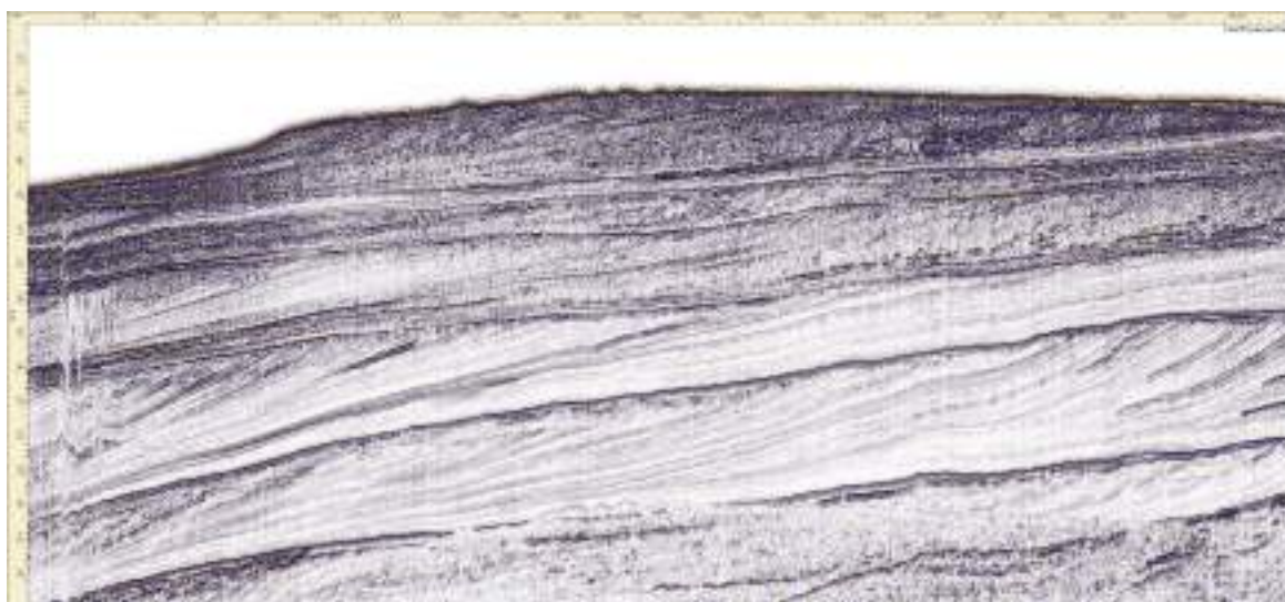
Figure 2-9: Zero-phase corrected final processed stack (Time-Variant Bandpass filter, FK filter, Gain balancing).
