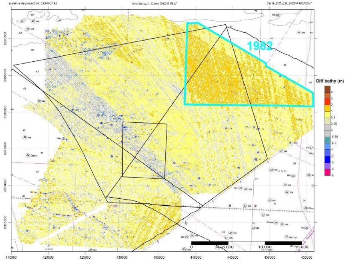
**Figure 3-1:** Bathymetric differentials 2020 to 1983 and 2020 to 1982.
