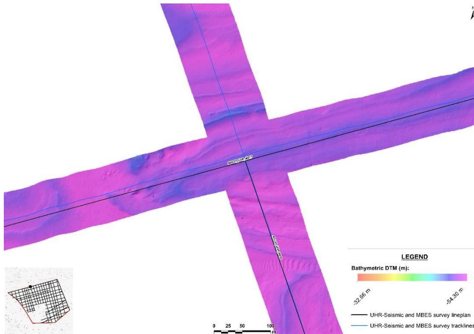
**Figure 3-8:** Detail of the bathymetric data grid model (0.5 x 0.5 m) for the Windfarm area of the NOR\_AO4 area – Lines AO4-21\_UHR\_M017 and – Lines AO4-21\_UHR\_X018.
