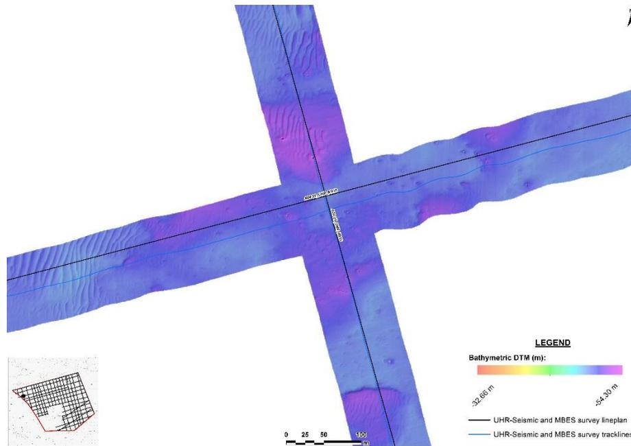
**Figure 3-4:** Detail of the bathymetric data grid model (0.5 x 0.5 m) for the Windfarm area of the NOR\_AO4 area – Lines AO4-21\_UHR\_M015 and – Lines AO4-21\_UHR\_X013.
