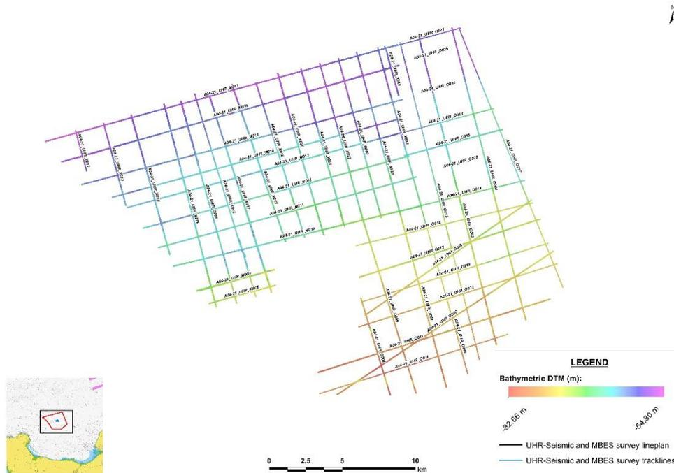
**Figure 3-3:** Whole bathymetric data grid model (0.5 x 0.5 m) for the Windfarm area of the NOR\_AO4 area.
