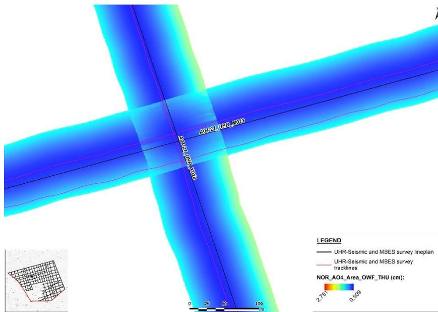
**Figure 3-10:** Example in detail of the results for the total horizontal uncertainty in the offshore windfarm of the NOR\_AO4 area.
