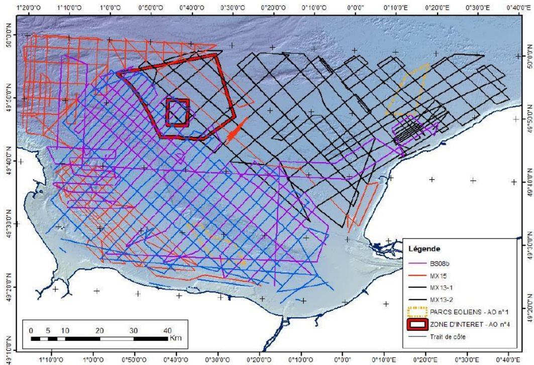
**Figure 3-13:** Map showing sparker seismic profiles of the four campaigns (Thinon & Serrano, 2021).
