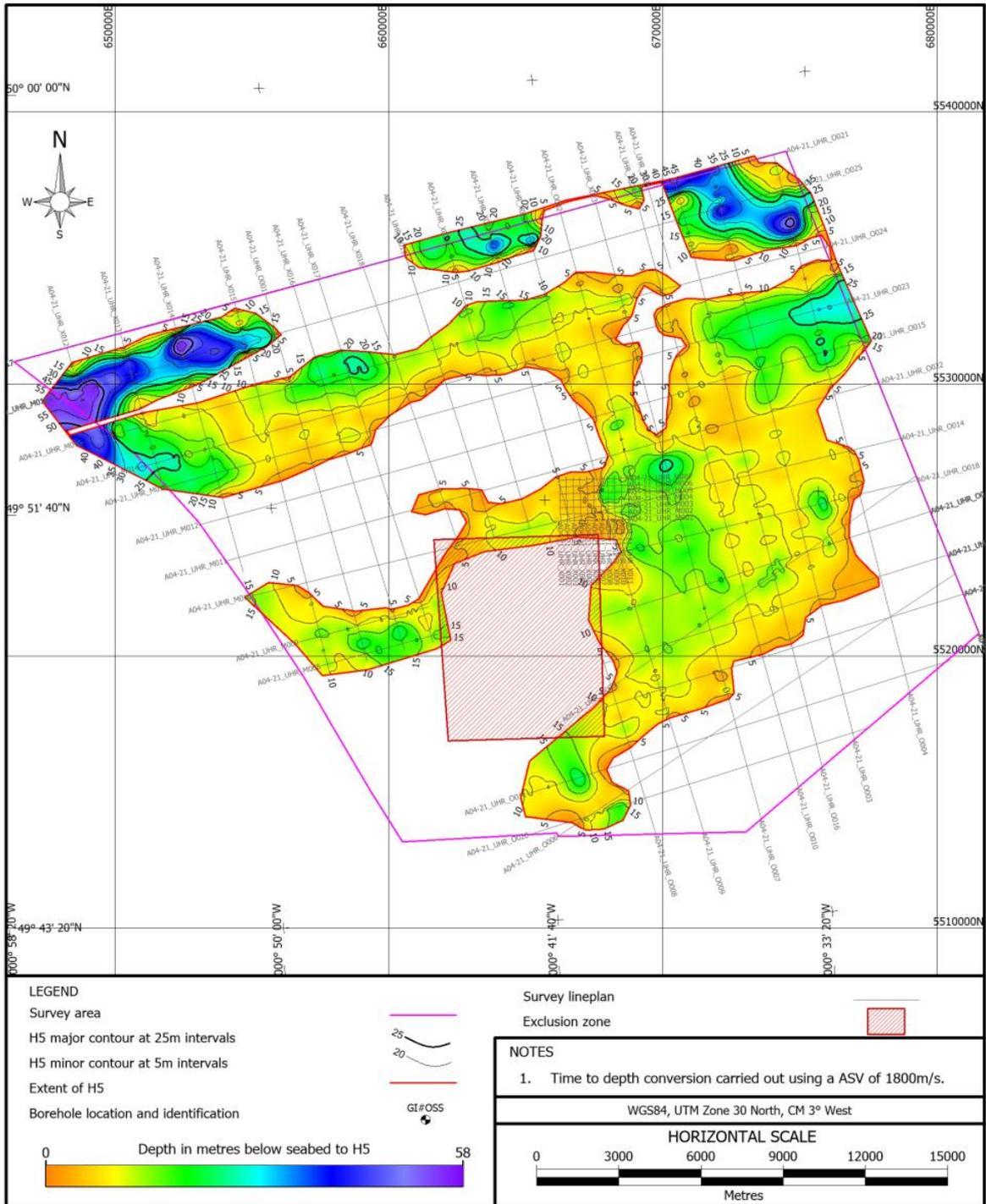
Figure 3-16: Isopach and extent of channel infill (H5)
