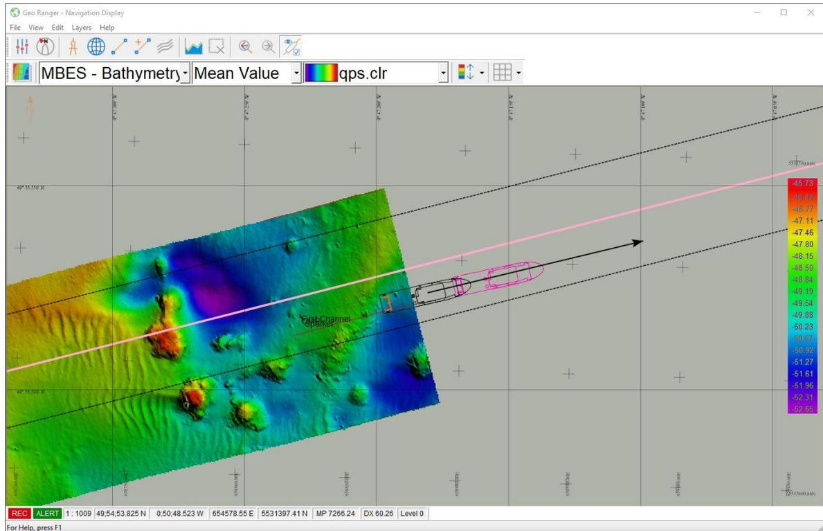
**Figure 2-1:** MBES bathymetry data acquisition with the QINSy software.
