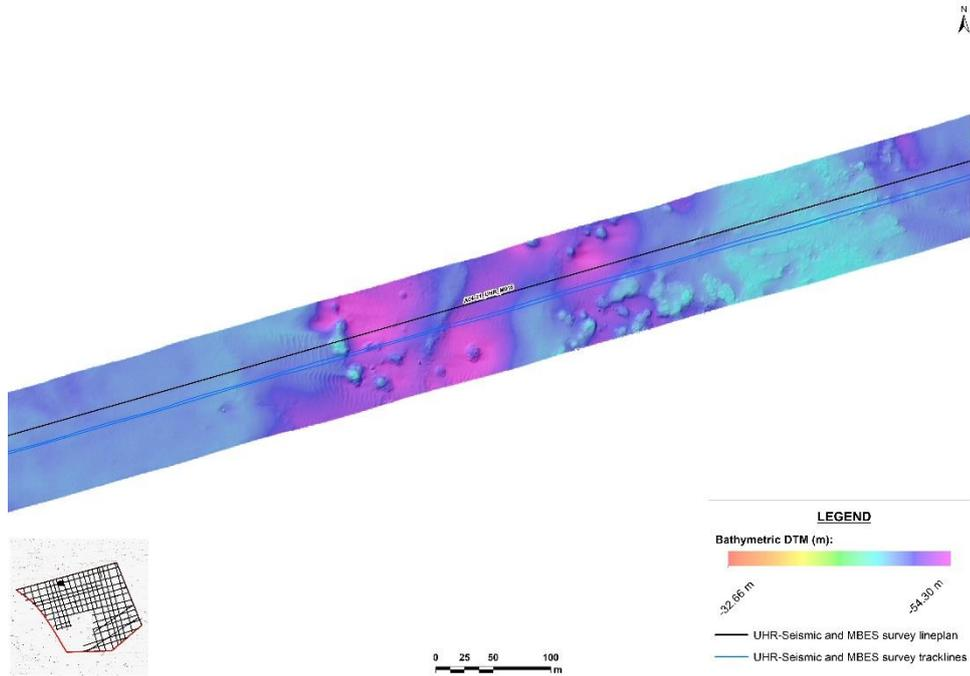
**Figure 3-6:** Detail of the bathymetric data grid model (0.5 x 0.5 m) for the Windfarm area of the NOR\_AO4 area – Line AO4-21\_UHR\_M016.
