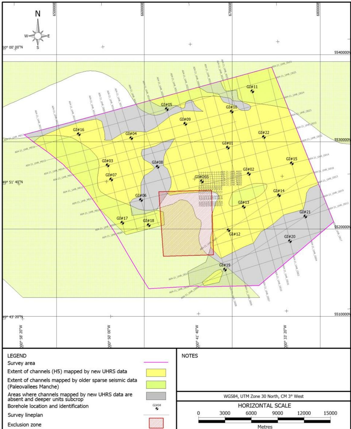
**Figure 3-17:** Extents of mapped channel infill (new UHR seismic vs older sparse seismic) related to planned boreholes.
