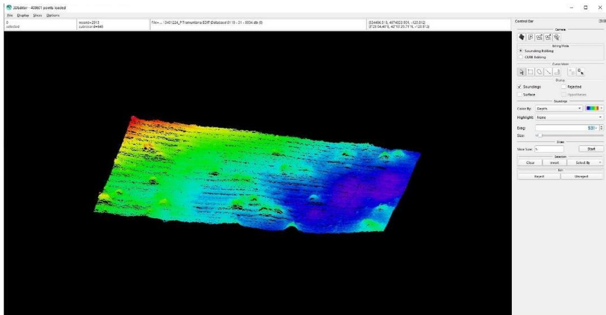
**Figure 2-3:** 3D image of the MBES bathymetry processing.
