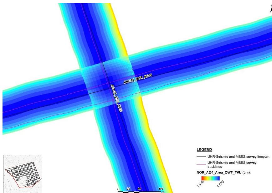
**Figure 3-12:** Example in detail of the results for the total vertical uncertainty in the offshore windfarm of the NOR\_AO4 area.
