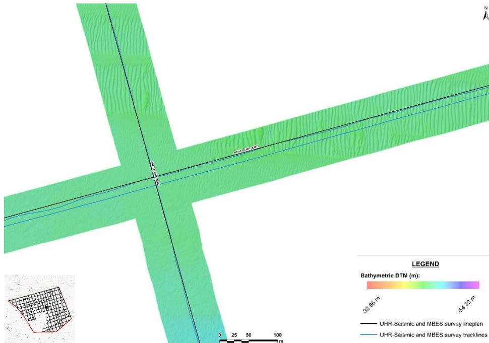
**Figure 3-7:** Detail of the bathymetric data grid model (0.5 x 0.5 m) for the Windfarm area of the NOR\_AO4 area – Lines AO4-21\_UHR\_M011 and – Lines AO4-21\_UHR\_X022.
