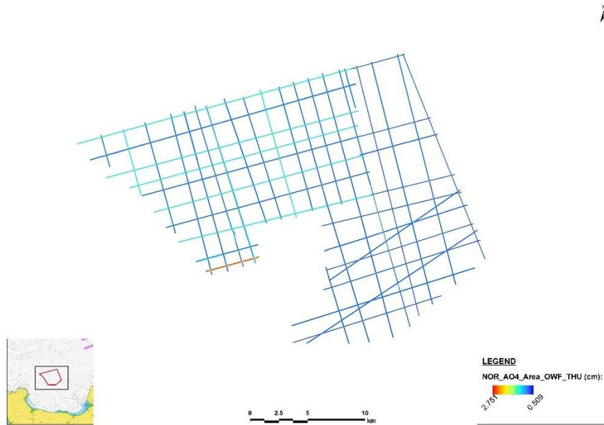
**Figure 3-9:** Results for the total horizontal uncertainty in the offshore windfarm of the NOR\_AO4 area – General.
