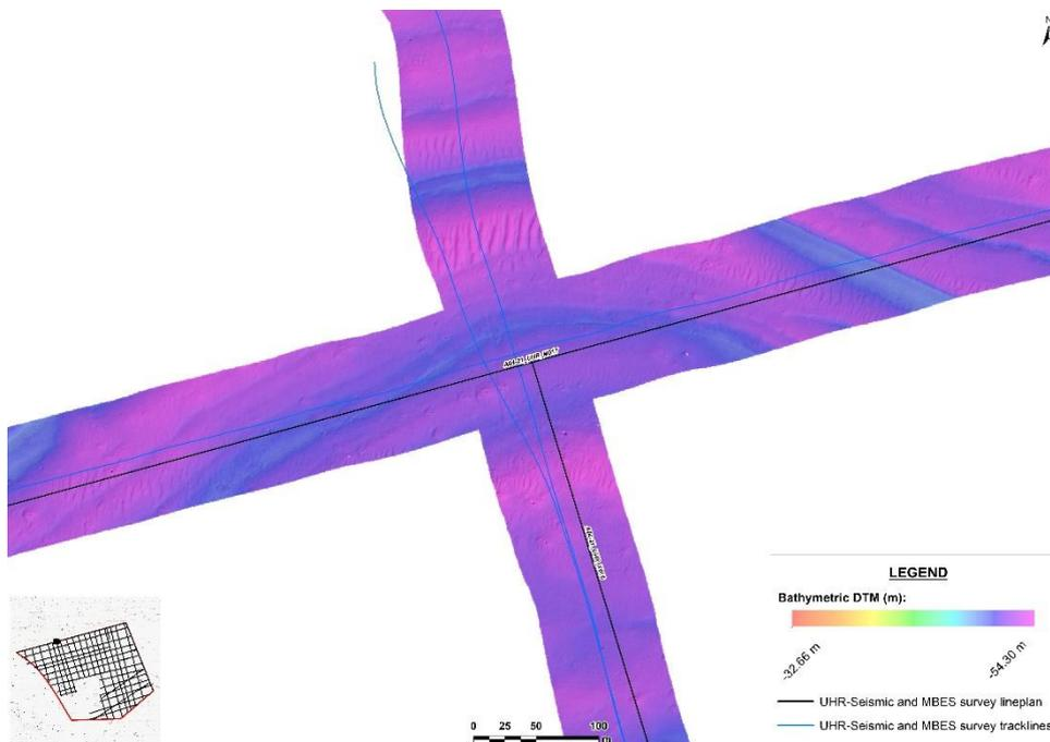
**Figure 3-5:** Detail of the bathymetric data grid model (0.5 x 0.5 m) for the Windfarm area of the NOR\_AO4 area – Lines AO4-21\_UHR\_M017 and – Lines AO4-21\_UHR\_X016.
