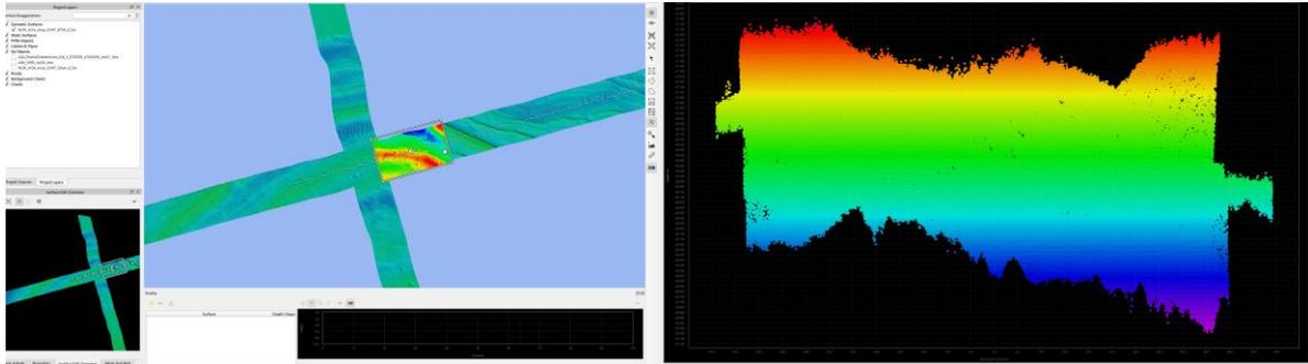
**Figure 2-2:** Processing screen of MBES bathymetry data with the Qimera software.
