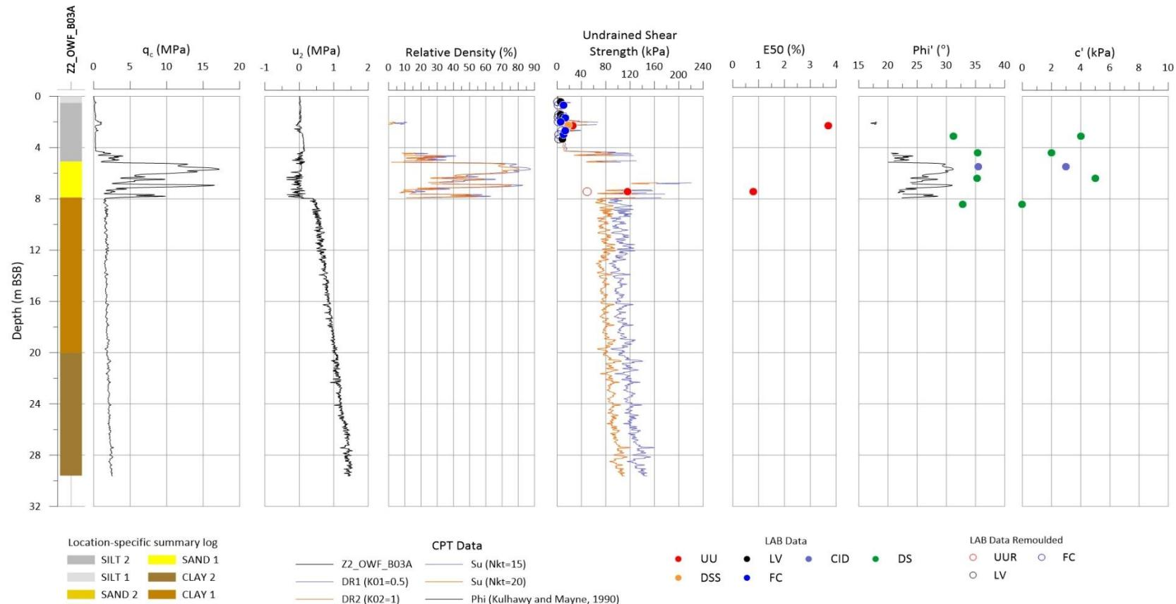
**Figure 11-3** qc, u<sub>2</sub>, relative density, Su, E50, Phi' and c' for Z2\_OWF\_B03A.
