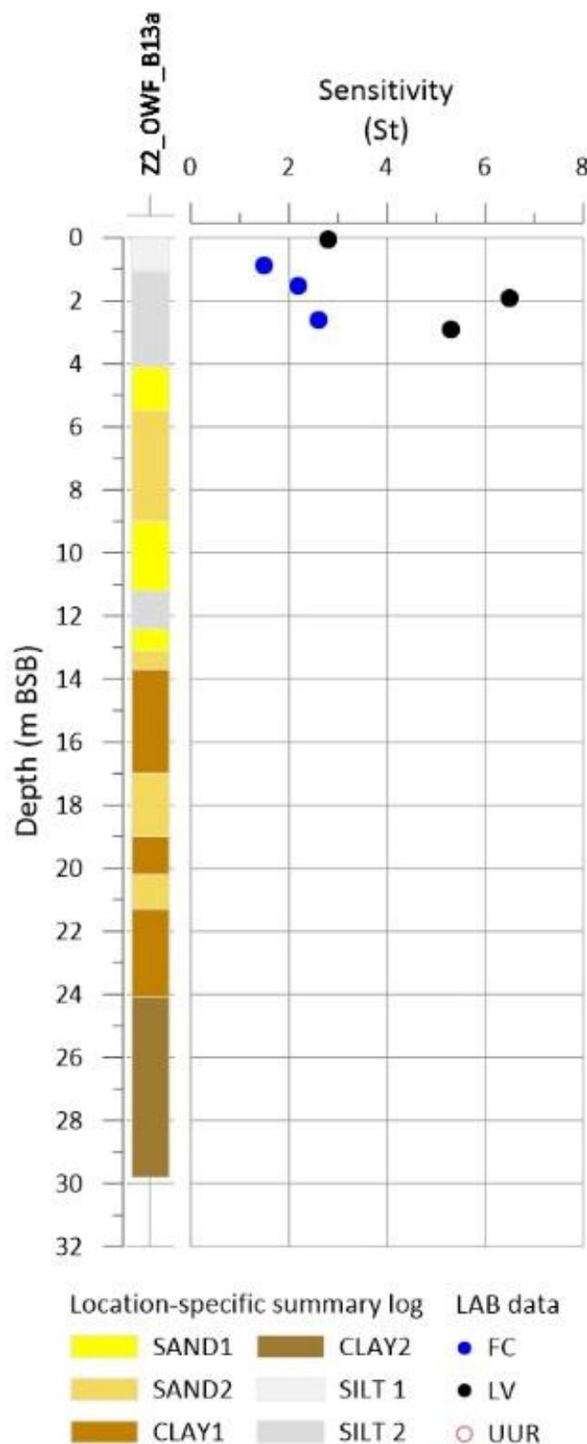
**Figure 11-28** Sensitivity for Z2\_OWF\_B13a.
