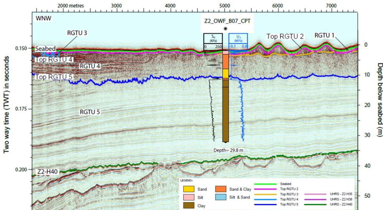
**Figure 6-5** Geotechnical location CPT B07 on UHRS on an WSW-ENE section.
