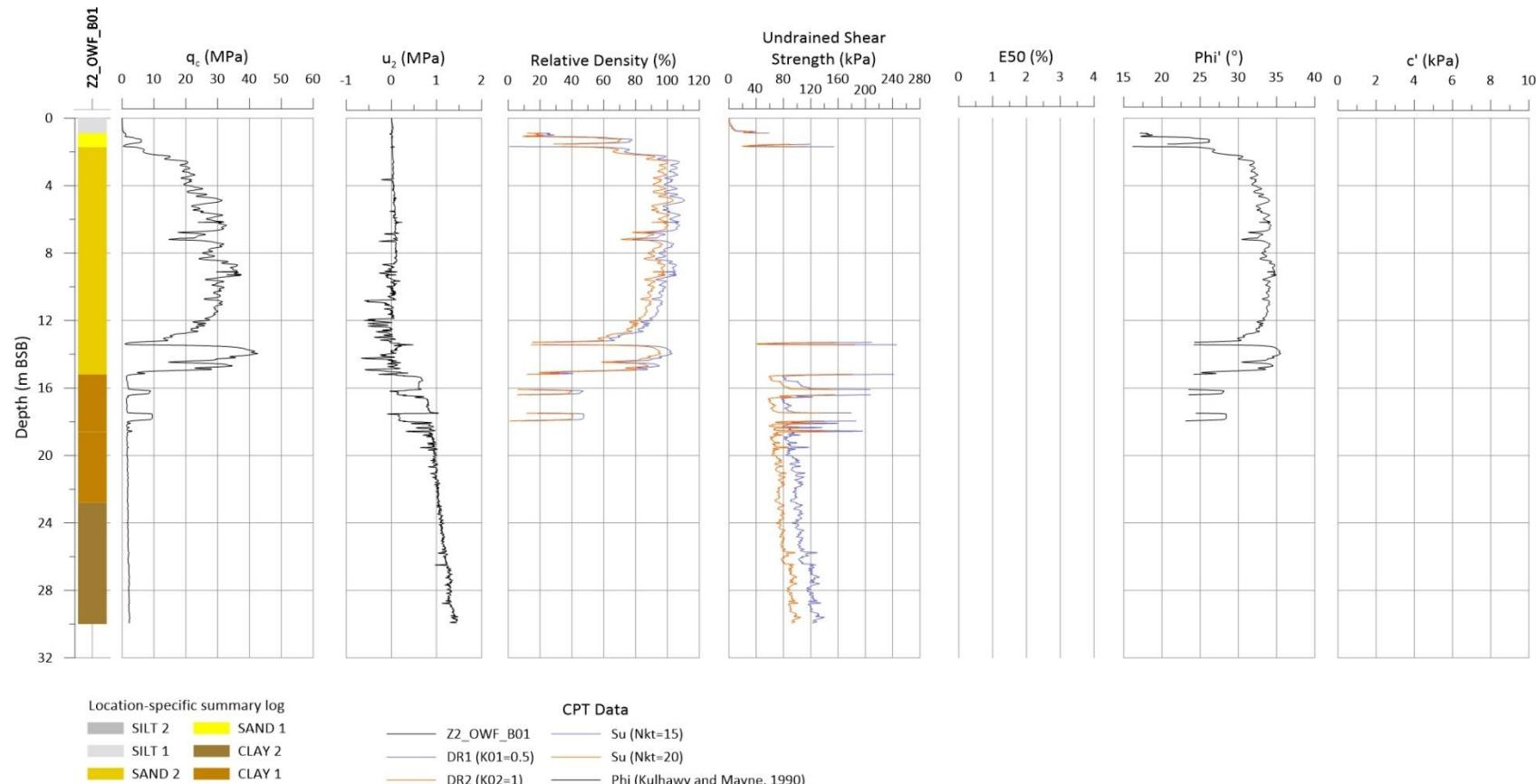
**Figure 11-1** qc, u2, relative density, Su, E50, Phi' and c' for Z2\_OWF\_B01.
