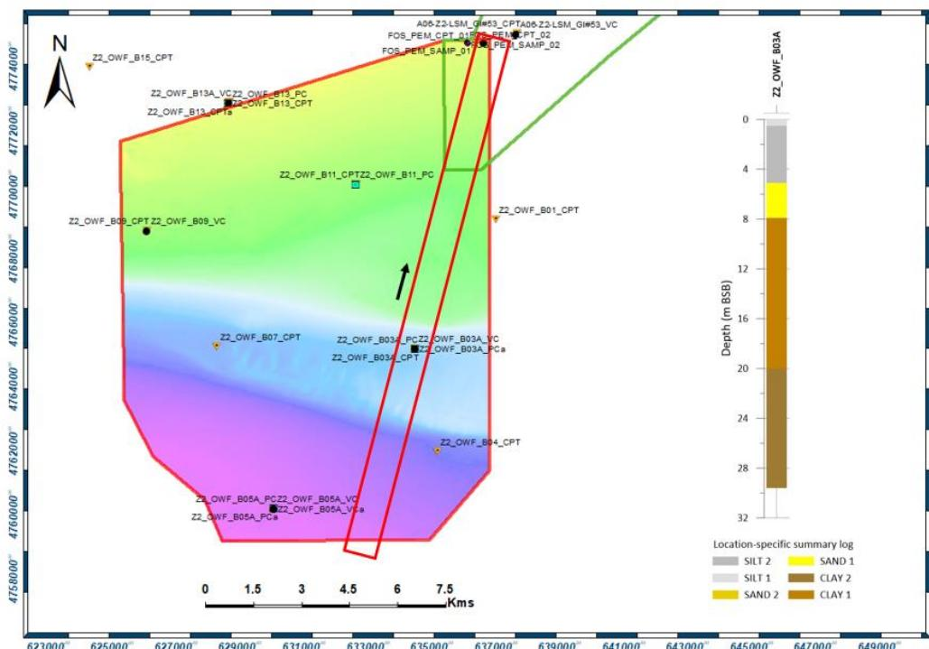
**Figure 10-4 Geotechnical Units within the CPT of Soil Profile 3.**
