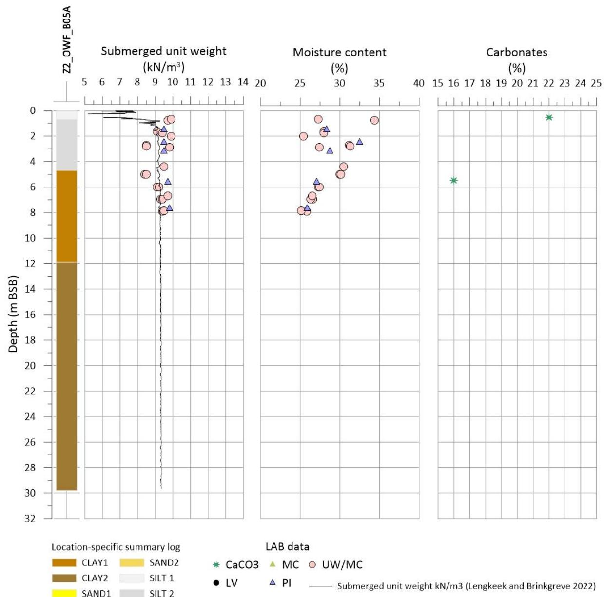
Figure 11-12 Submerged unit weight, moisture content and Carbonate content for Z2\_OWF\_B05A.
