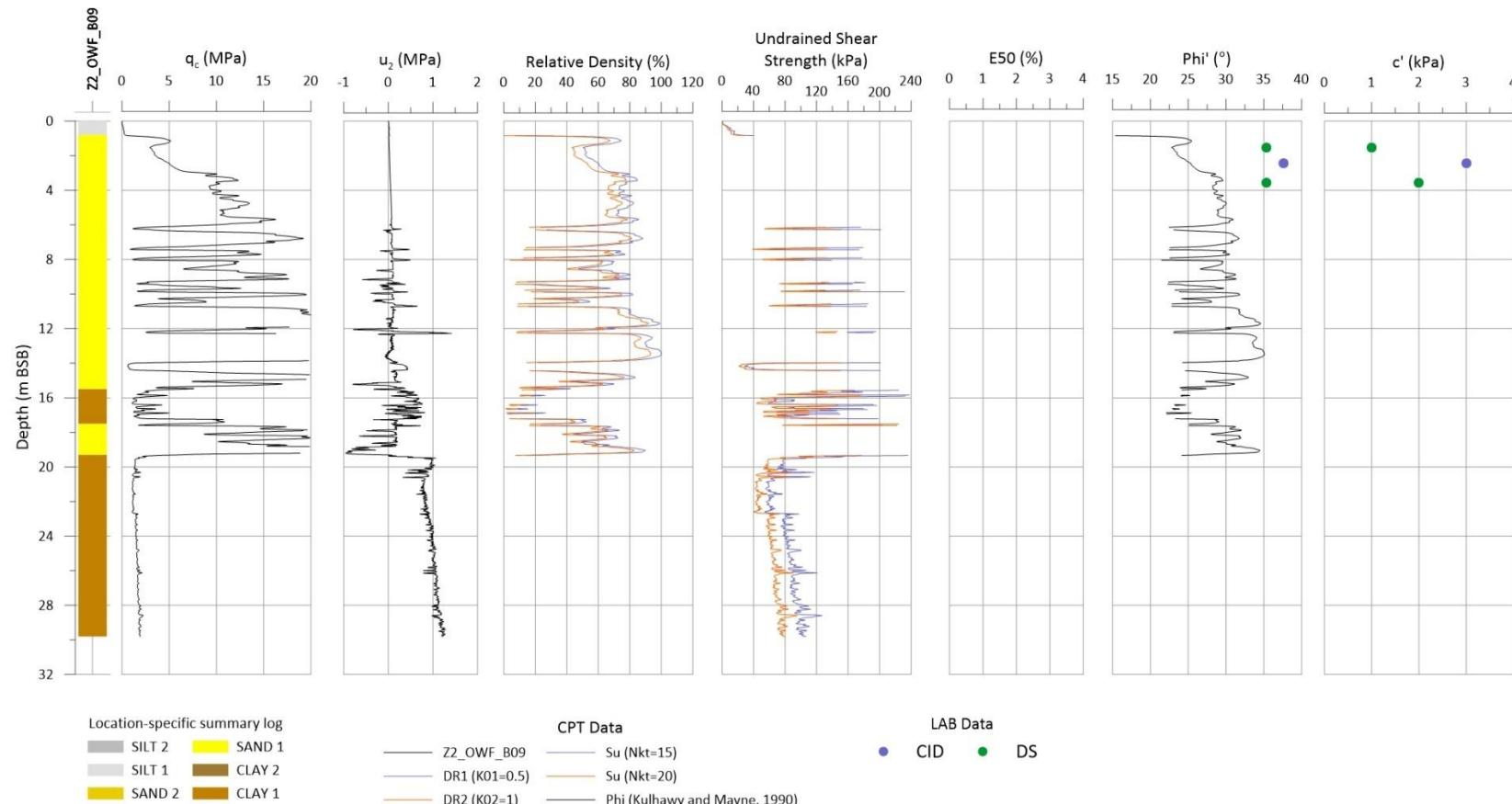
Figure 11-17 qc,  $u_2$ , relative density,  $S_u$ ,  $E_{50}$ ,  $\Phi'_i$  and  $c'$  for Z2\_OWF\_B09.
