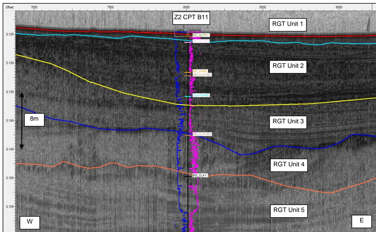
**Figure 6-3** Geotechnical location CPT B11 on SHOM SBP data.
