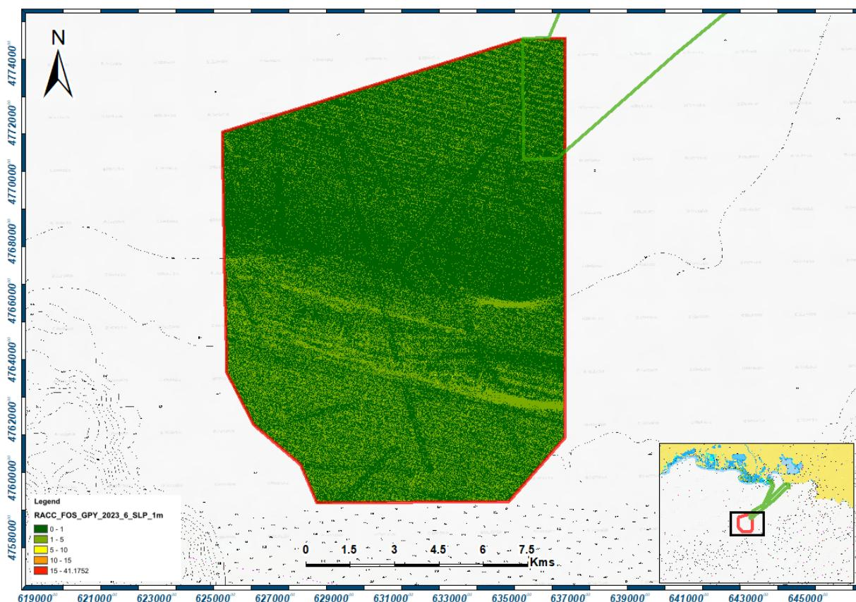
**Figure 7-3** Slope map from AO6 OWF area. Slope raster calculated from the SHOM bathymetry raster, with 1 x 1 m pixel resolution.
