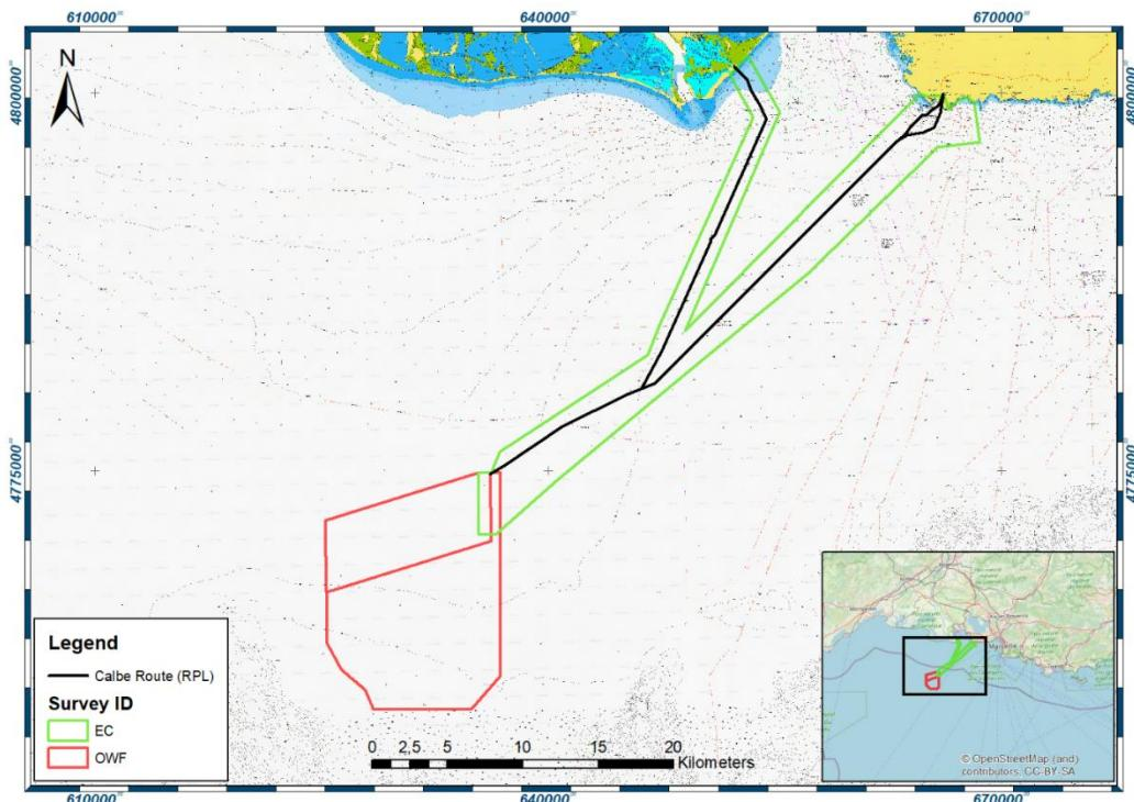
**Figure 1-1** AO6 Windfarm area (OWF) and Export cable (EC) in the MED\_AO6 Survey area.
