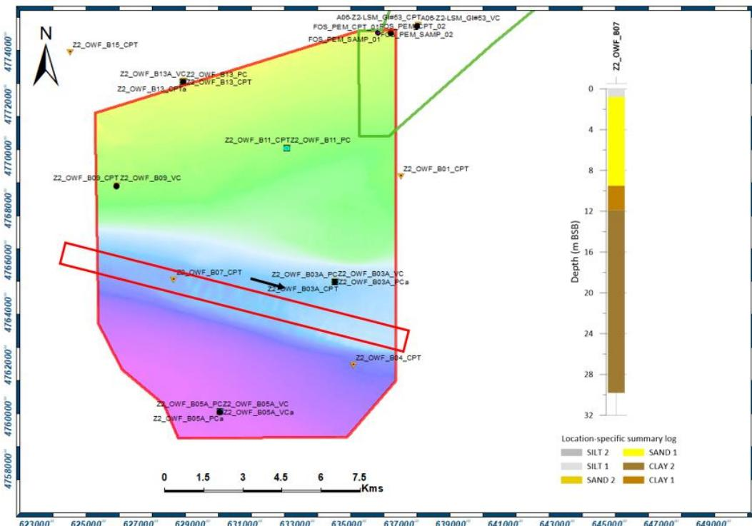
Figure 10-6 Geotechnical Units within the CPT of Soil Profile 5.
