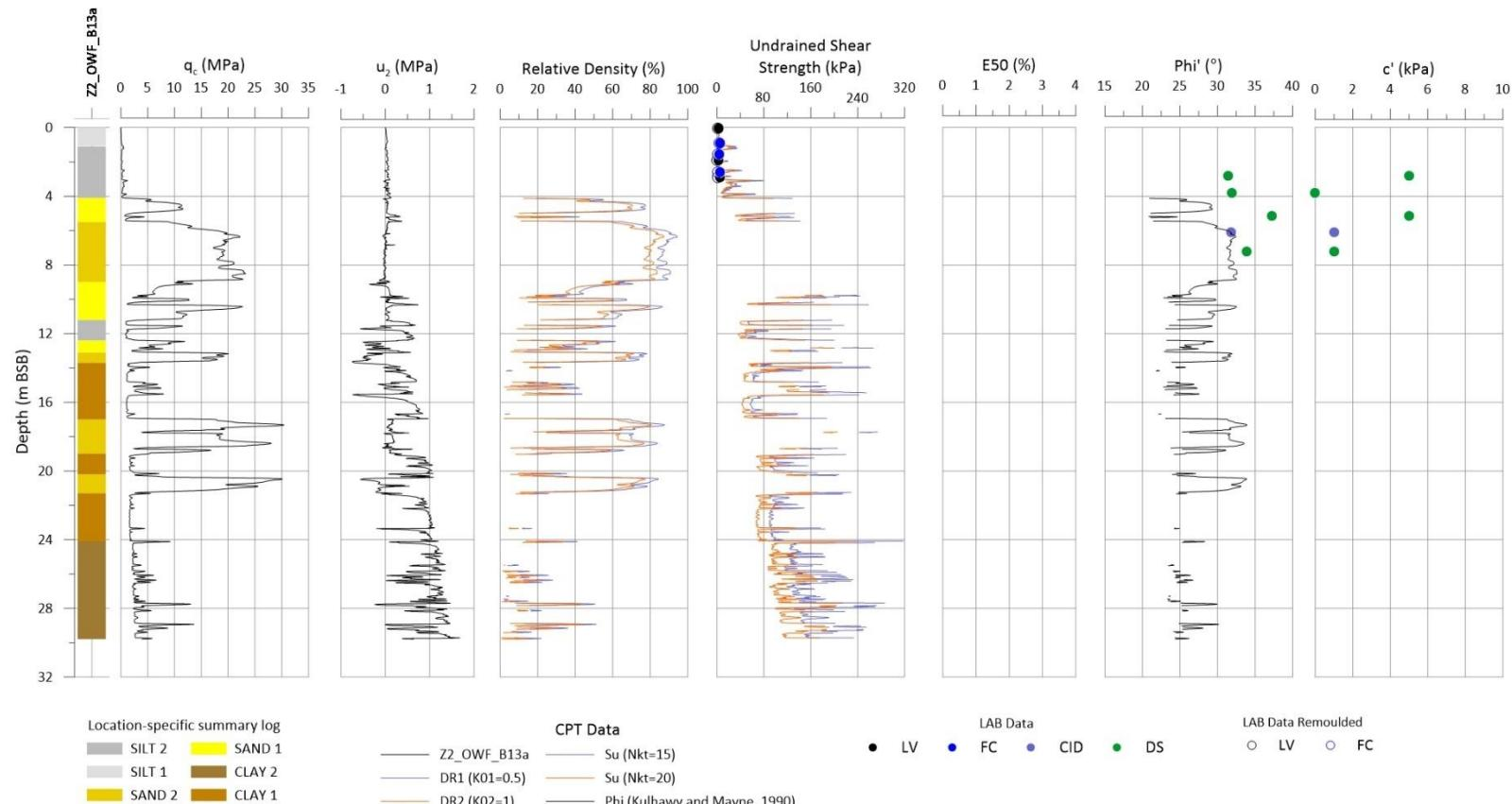
Figure 11-24 qc, u<sub>2</sub>, relative density, Su, E50, Phi' and c' for Z2\_OWF\_B13a.
