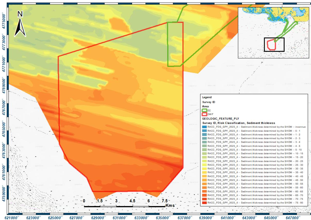
**Figure 4-4** AO6 – OWF Zone 2 SHOM SBP sediment thickness map with sediment ranges in meters BSB of the Acoustic Basement (AB) (SHOM, 2022 (Ref. 14)).
