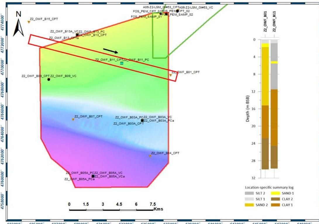
Figure 10-7 Geotechnical Units within the CPT of Soil Profile 6.
