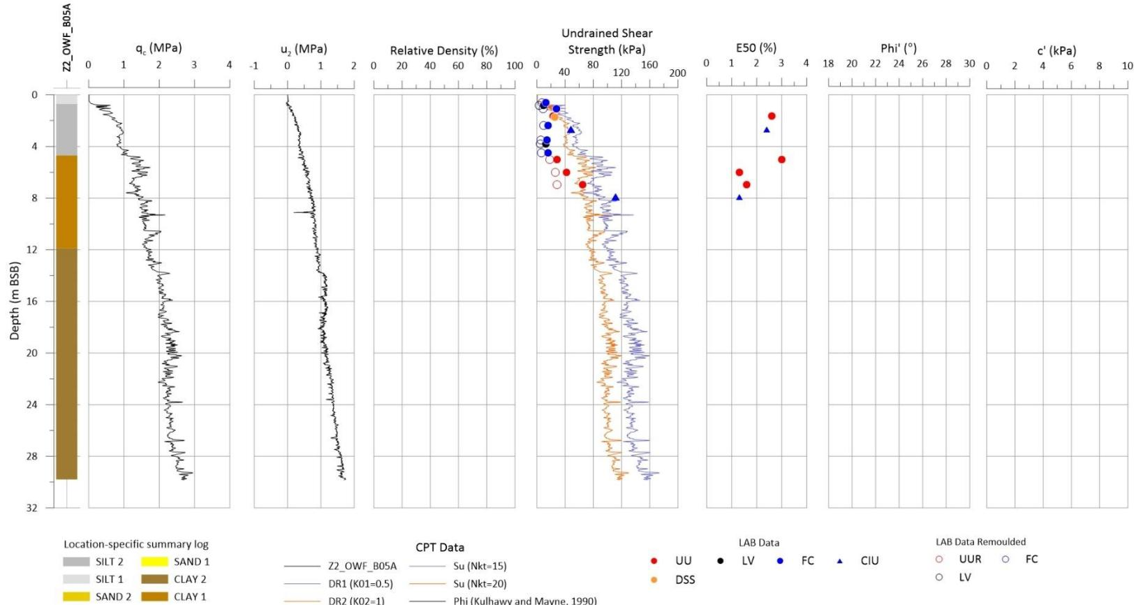
**Figure 11-10** qc, u<sub>2</sub>, relative density, Su, E50, Phi' and c' for Z2\_OWF\_B05A.
