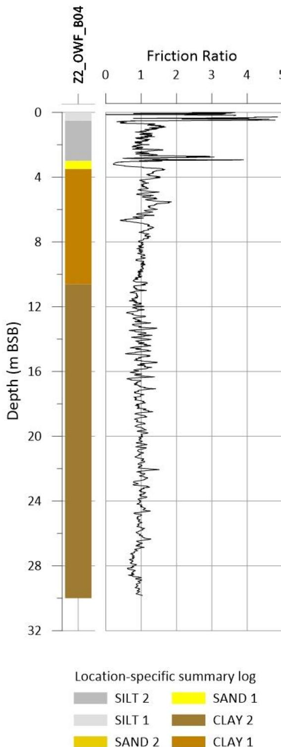
**Figure 11-9** Friction ratio for Z2\_OWF\_B04.
