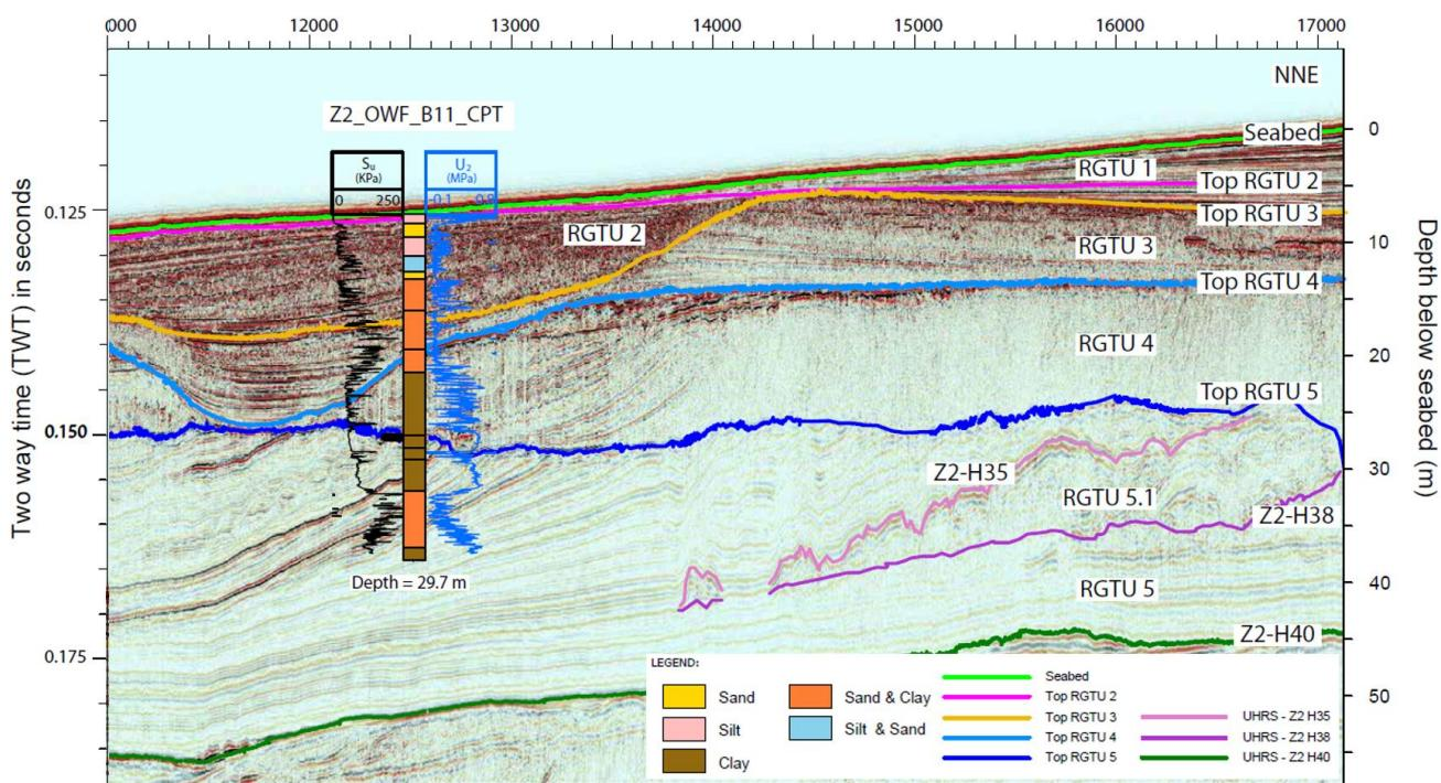
Figure 6-4 Geotechnical location CPT B11 on UHRS on an SSW-NNE section.
