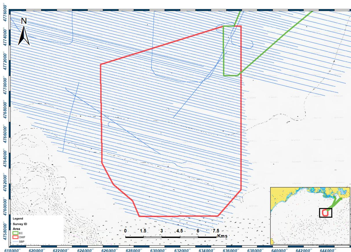
**Figure 4-3** Distribution map of SBP profiles track-lines acquired by SHOM in the AO6 OWF Zone 2 area
