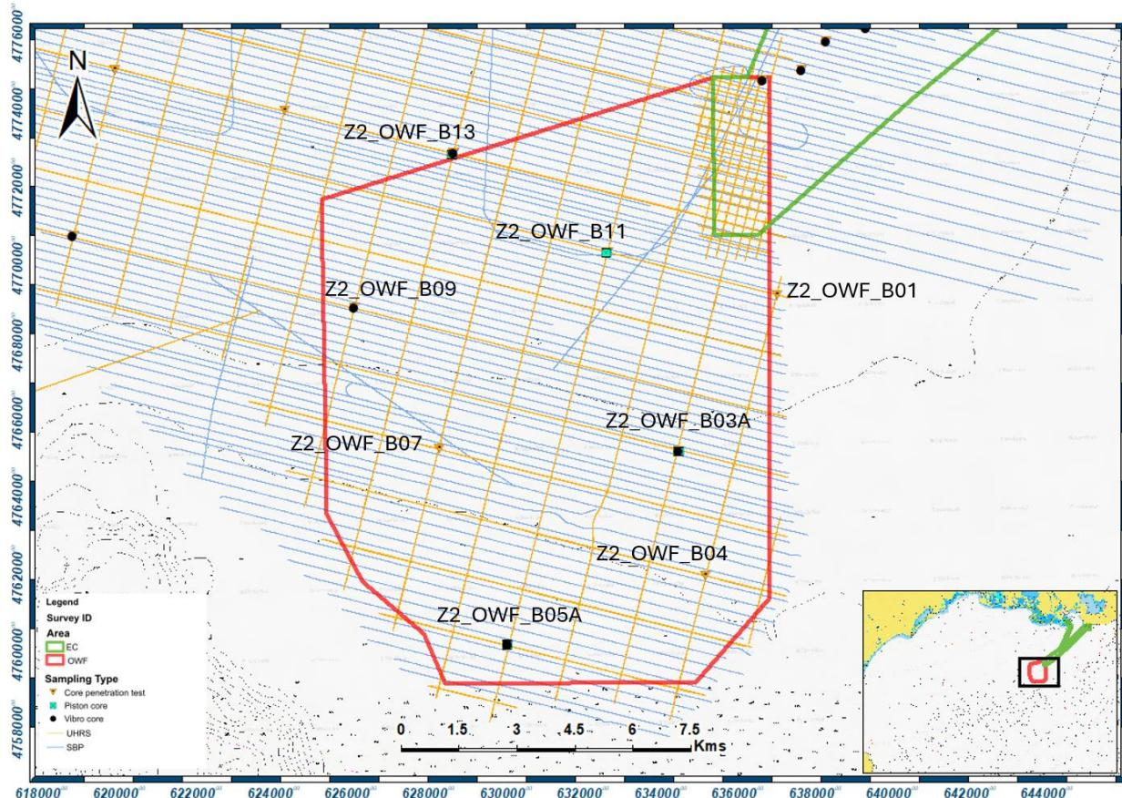
**Figure 6-2** Location of the geotechnical investigated sites within the OWF area. UHRS seismic profiles track-lines are shown in orange and SBP track-lines in blue colored lines.
