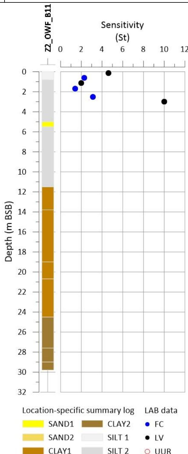
**Figure 11-23** Sensitivity for Z2\_OWF\_B11.
