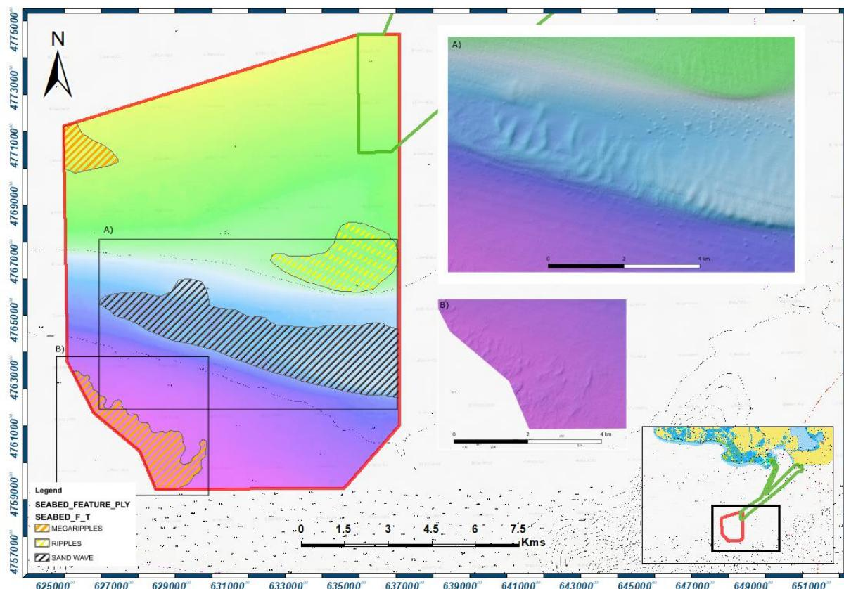
**Figure 7-7** Magnified view of mega ripples and ripples in the center area of the OWF.
