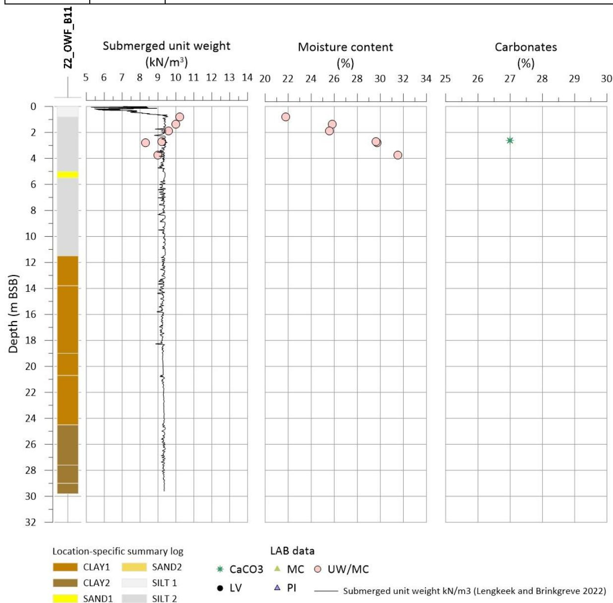
**Figure 11-22** Submerged unit weight, moisture content and Carbonate content for Z2\_OWF\_B11.
