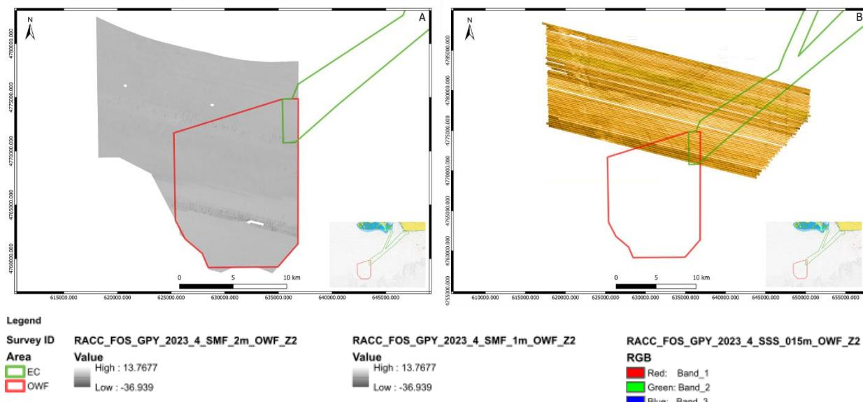
**Figure 4-2 SHOM's OWF a) MBES backscatter and b) SSS data.**
