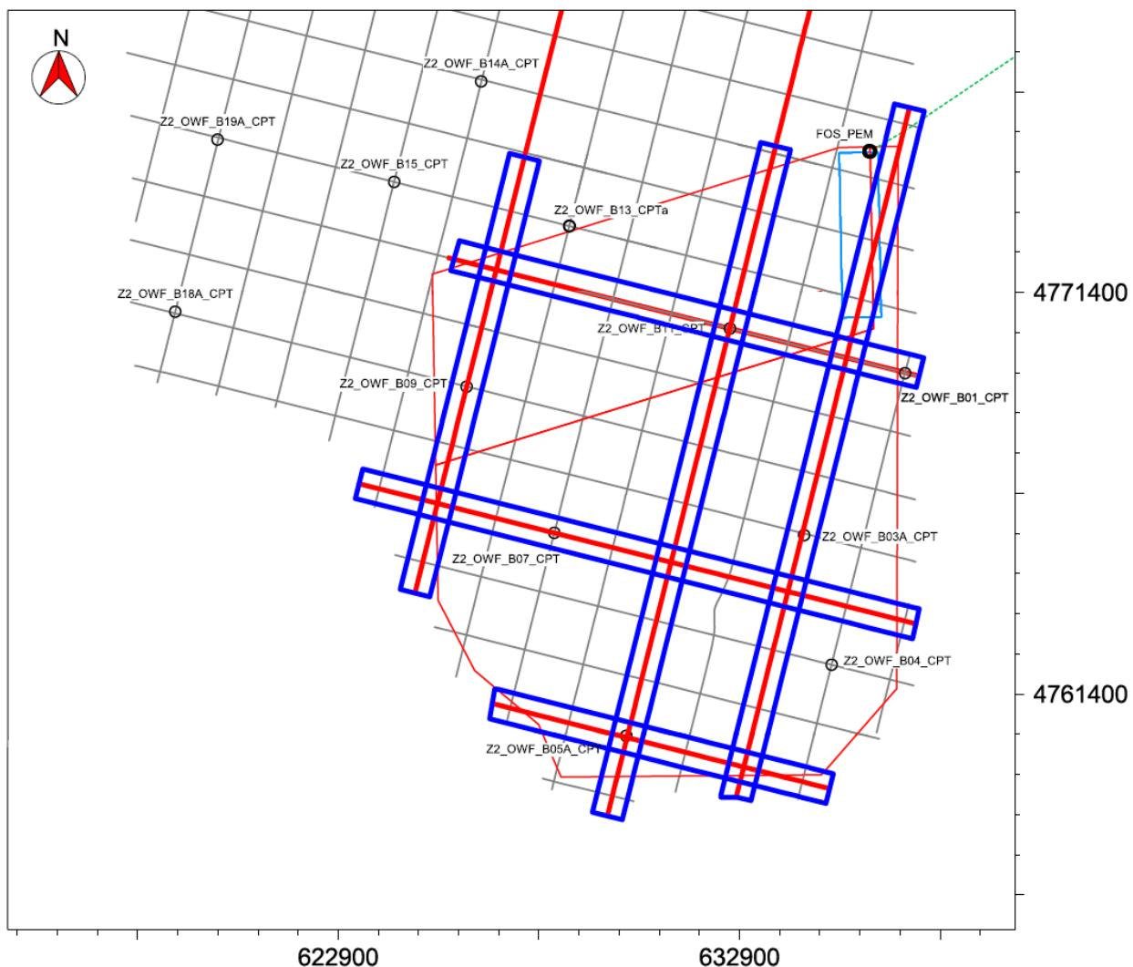
**Figure 6-6** UHRS lines selected for depicting the seismic regional profiles.
