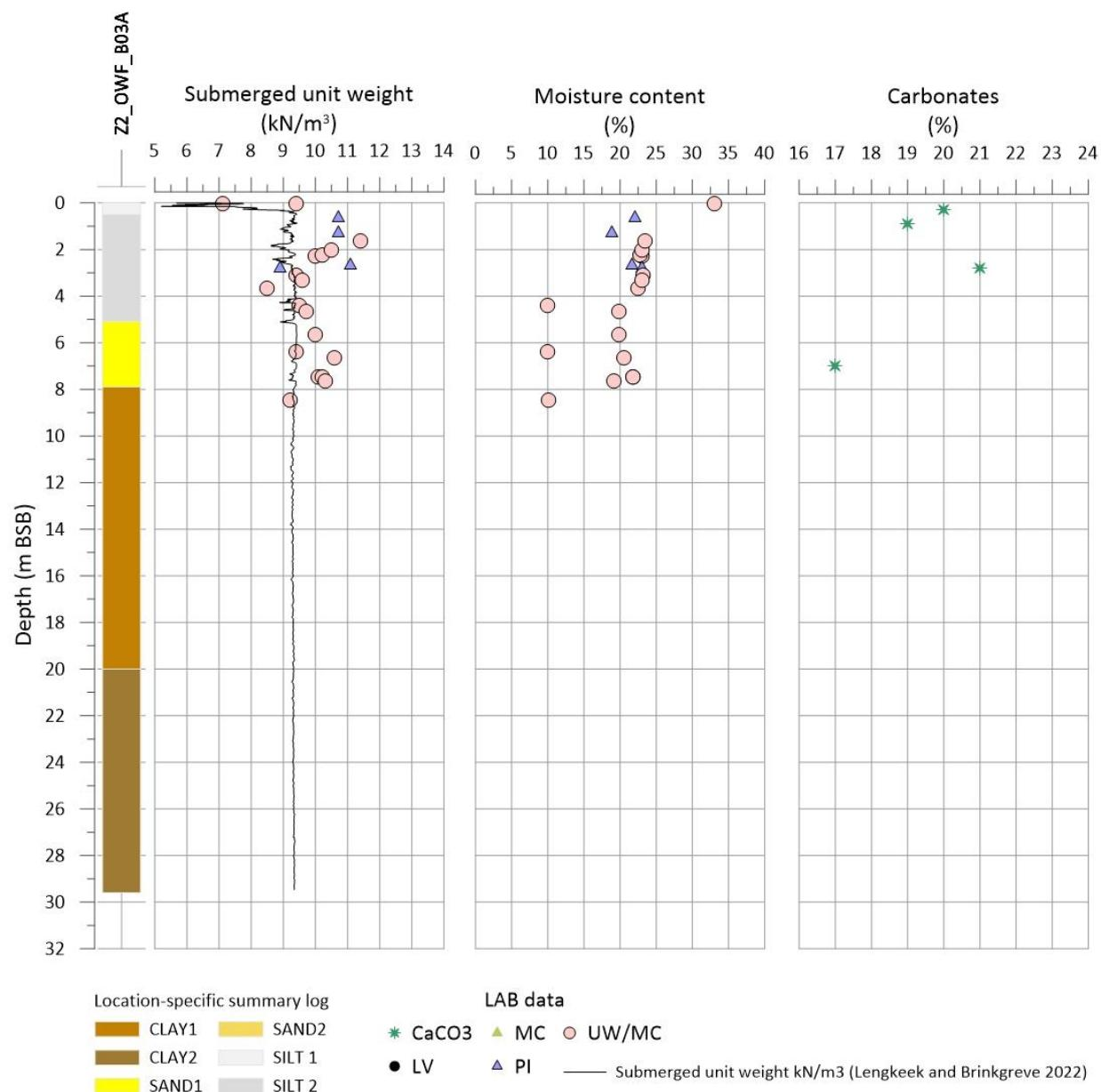
**Figure 11-4** Submerged unit weight, moisture content and Carbonate content for location Z2\_OWF\_B03A.
