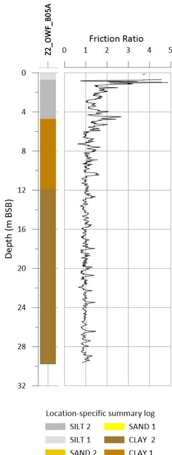
**Figure 11-11 Friction ratio for Z2\_OWF\_B05A.**
