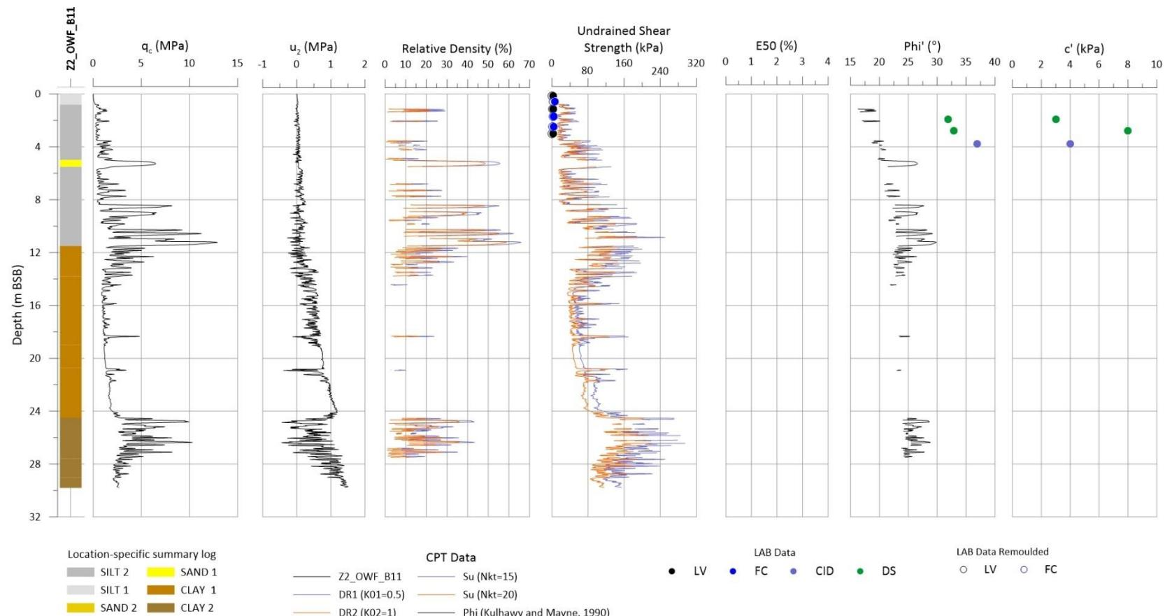
Figure 11-20 qc,  $u_2$ , relative density,  $S_u$ ,  $E_{50}$ ,  $\Phi'_i$  and  $c'$  for Z2\_OWF\_B11.
