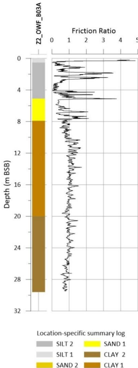
**Figure 11-5** Friction ratio for Z2\_OWF\_B03A.
