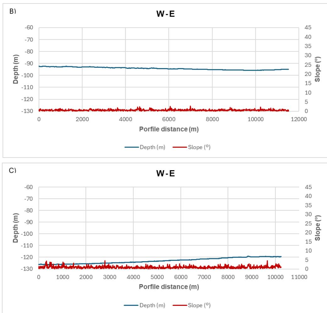
**Figure 7-2** Profiles a), b) and c) with the bathymetry as the blue line and the slope as the red one. The locations of these profiles can be found in Figure 7-1.
