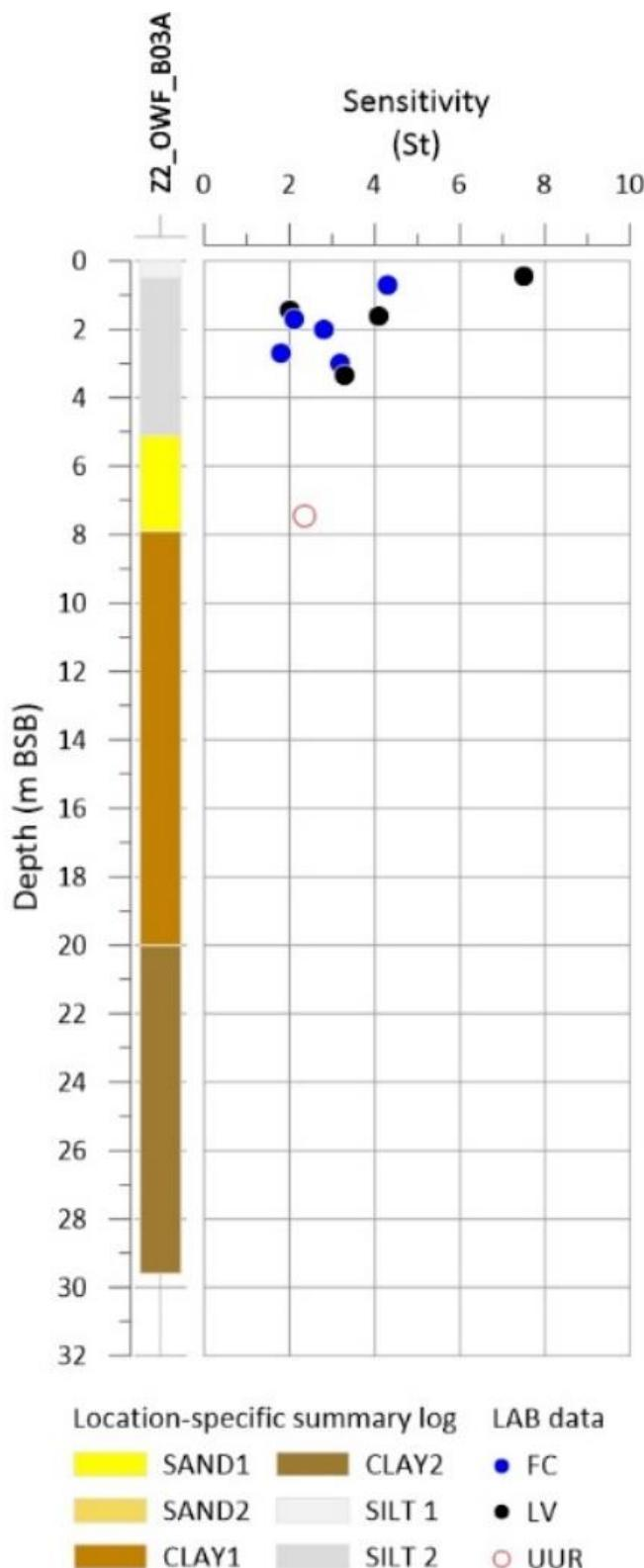
**Figure 11-7 Sensitivity for Z2\_OWF\_B03A.**
