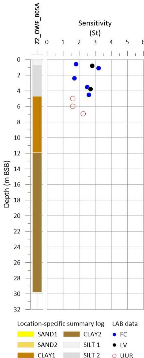
**Figure 11-14** Sensitivity for Z2\_OWF\_B05A.
