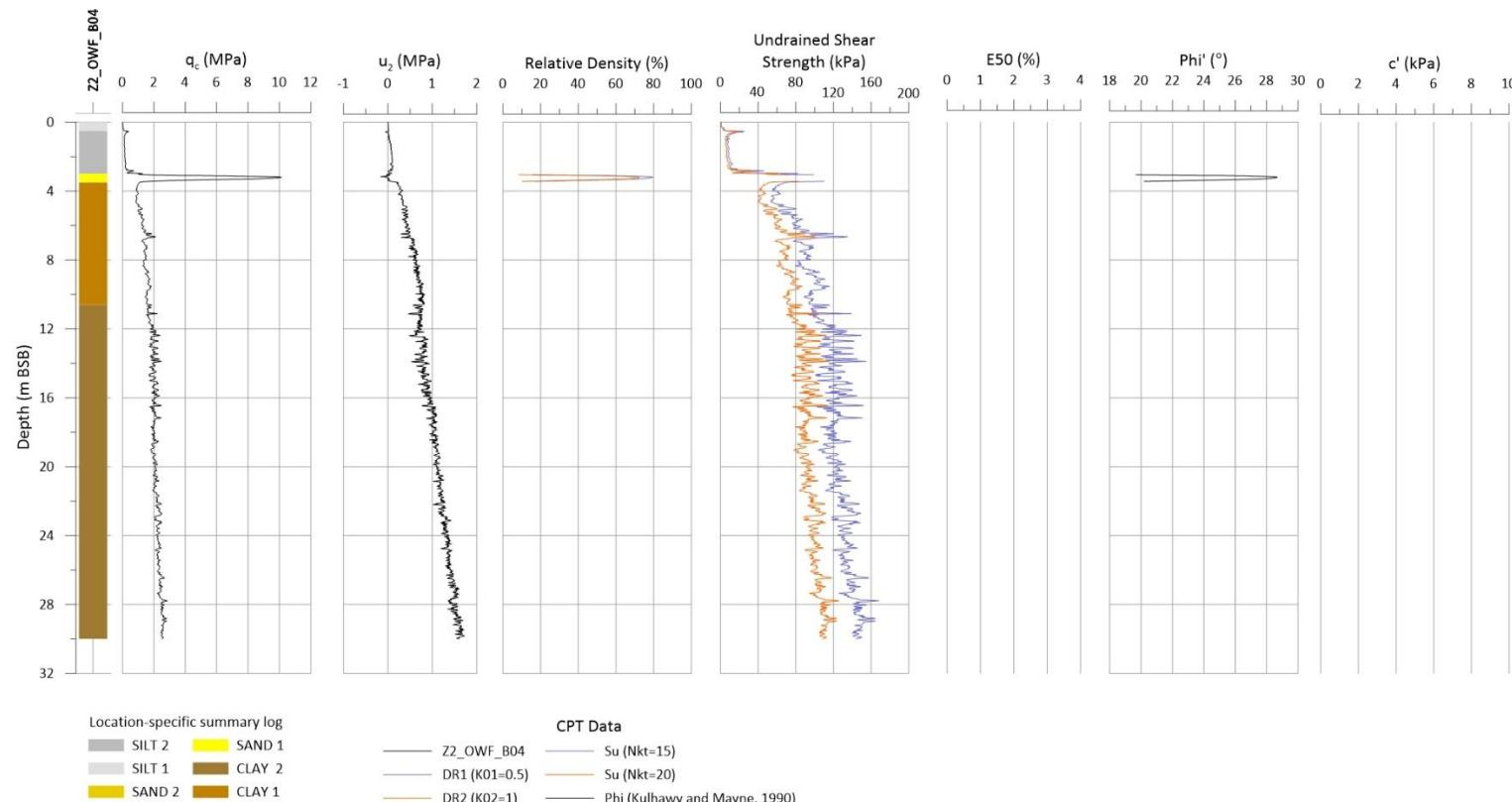
**Figure 11-8 qc, u<sub>2</sub>, relative density, Su, E50, Phi' and c' for Z2\_OWF\_B04.**
