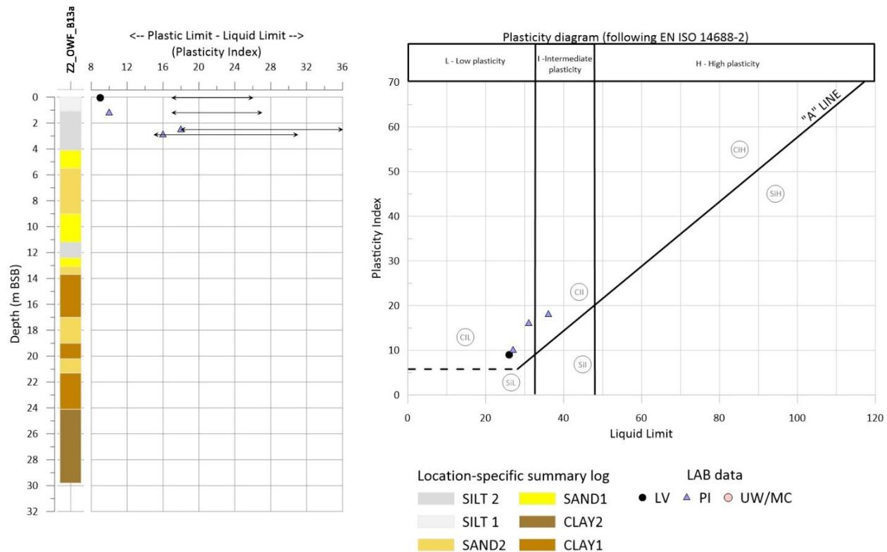
**Figure 11-27** Plasticity for Z2\_OWF\_B13a.
