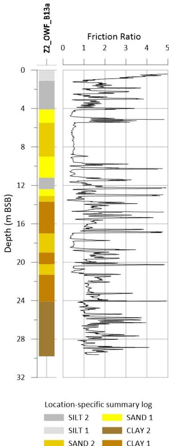
**Figure 11-25** Friction ratio for Z2\_OWF\_B13a.
