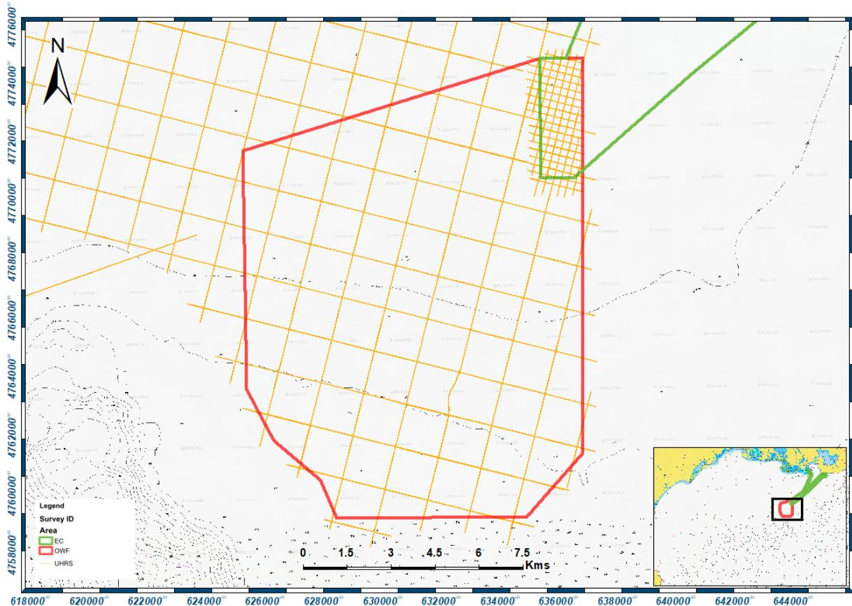
**Figure 4-5 UHRS Line plan for MED\_AO6 windfarm area (OWF).**
