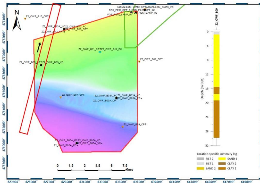
**Figure 10-2 Geotechnical Units within the CPT of Soil Profile 1.**
