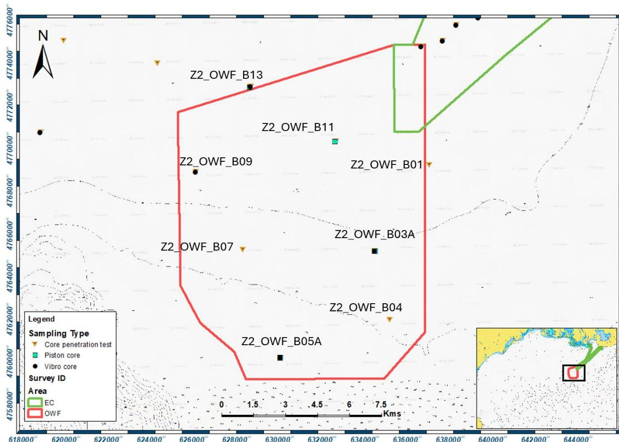
**Figure 4-8 Geotechnical sample points of AO6 FOS OWF 2.**
