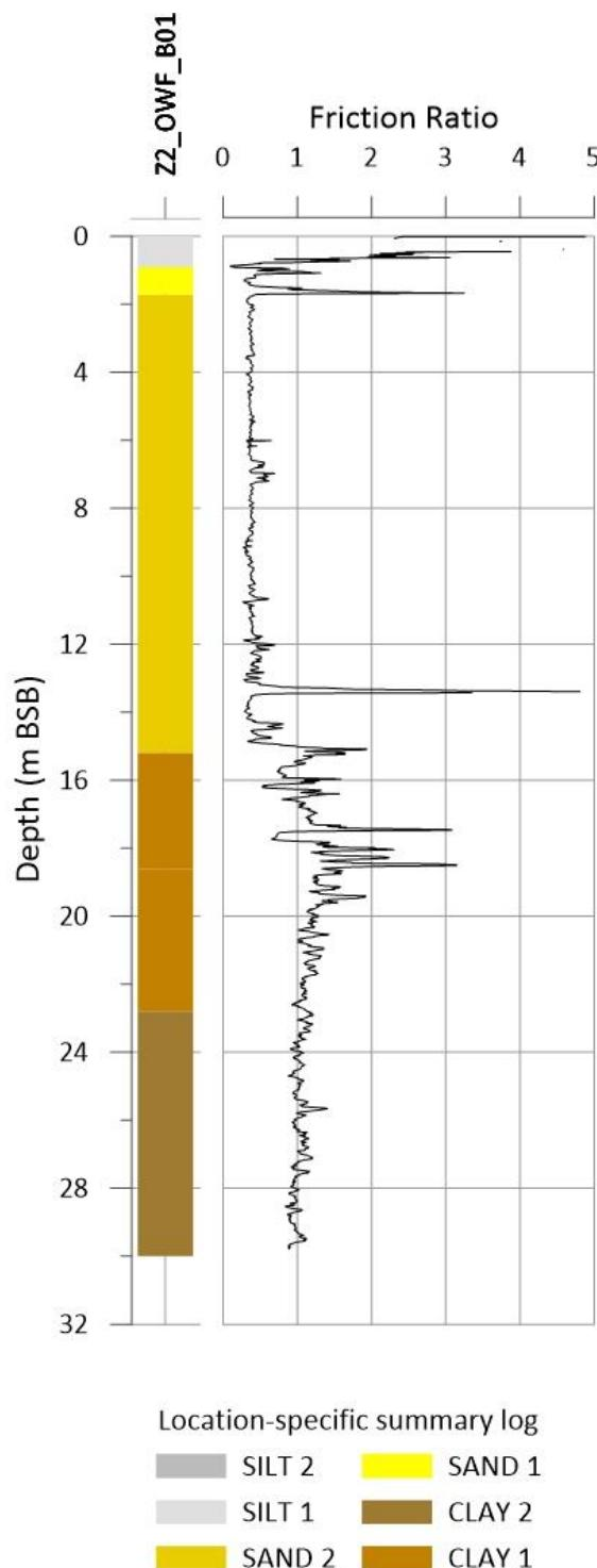
**Figure 11-2** Friction ratio for Z2\_OWF\_B01.
