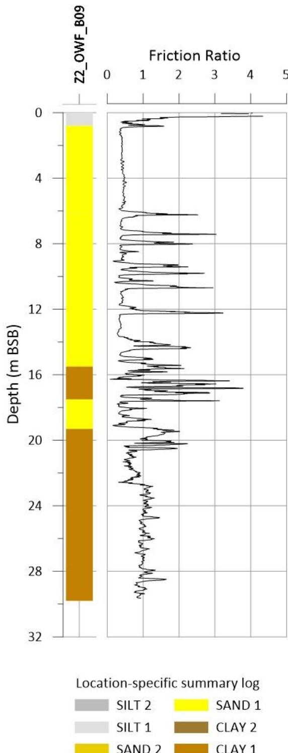
**Figure 11-18** Friction ratio Z2\_OWF\_B09.
