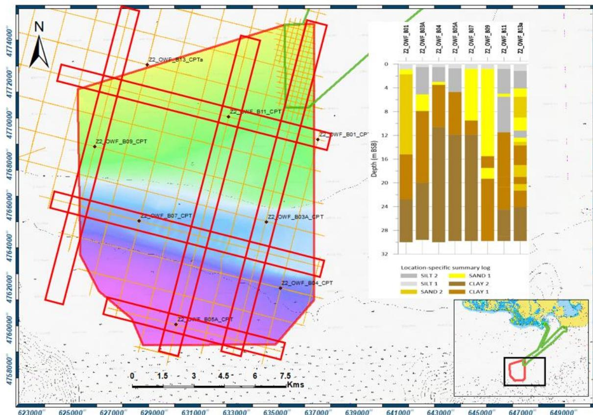
**Figure 10-1 Geotechnical Units AO6 OWF Z2.**
