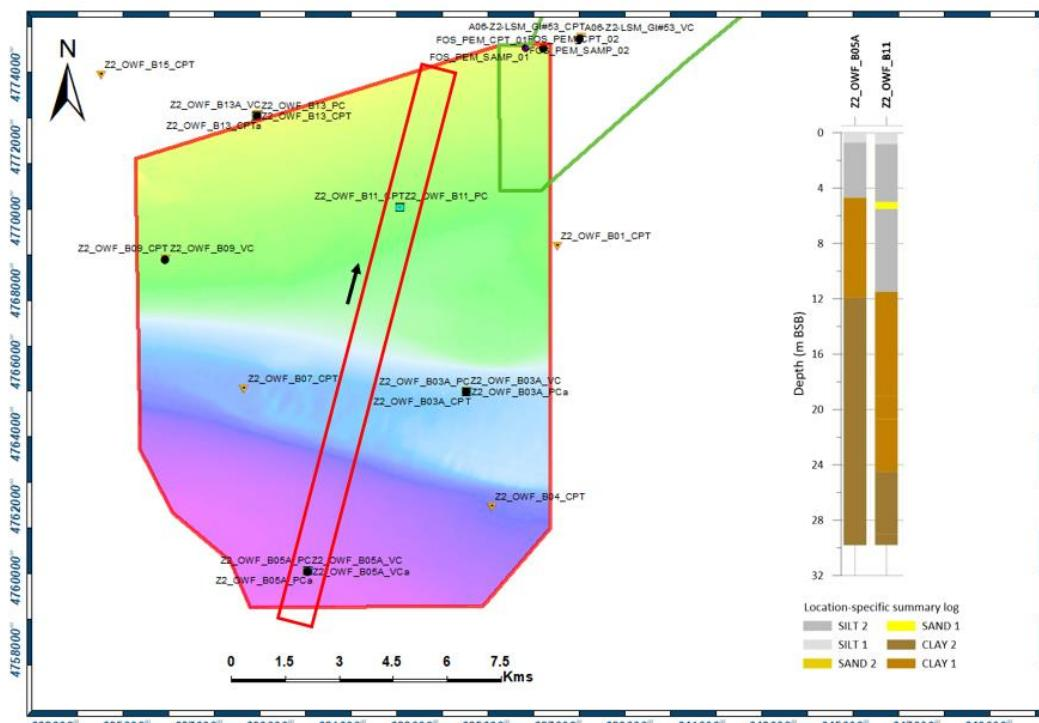
**Figure 10-3 Geotechnical Units within the CPT of Soil Profile 2.**
