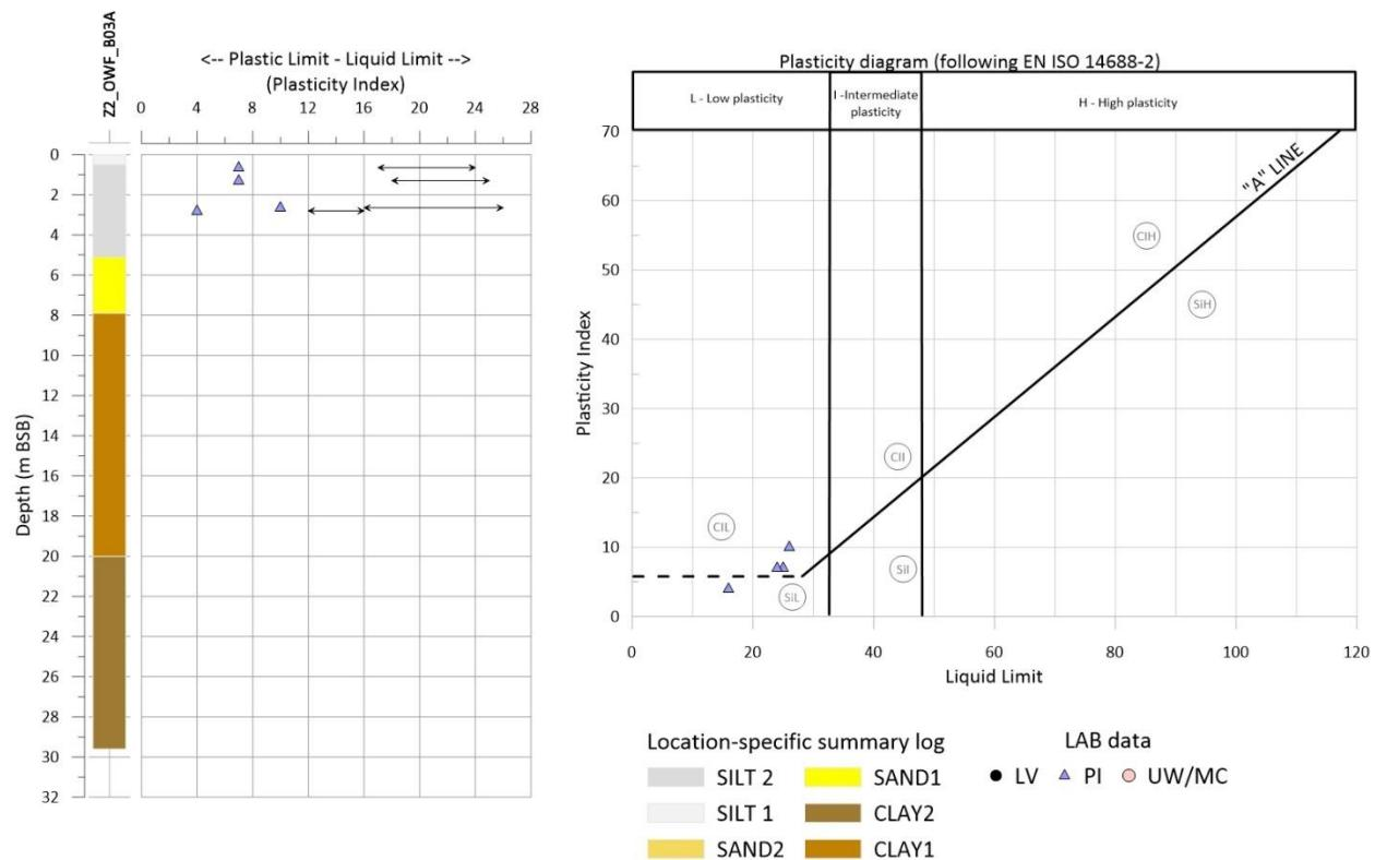
**Figure 11-6** Plasticity for Z2\_OWF\_B03A.
