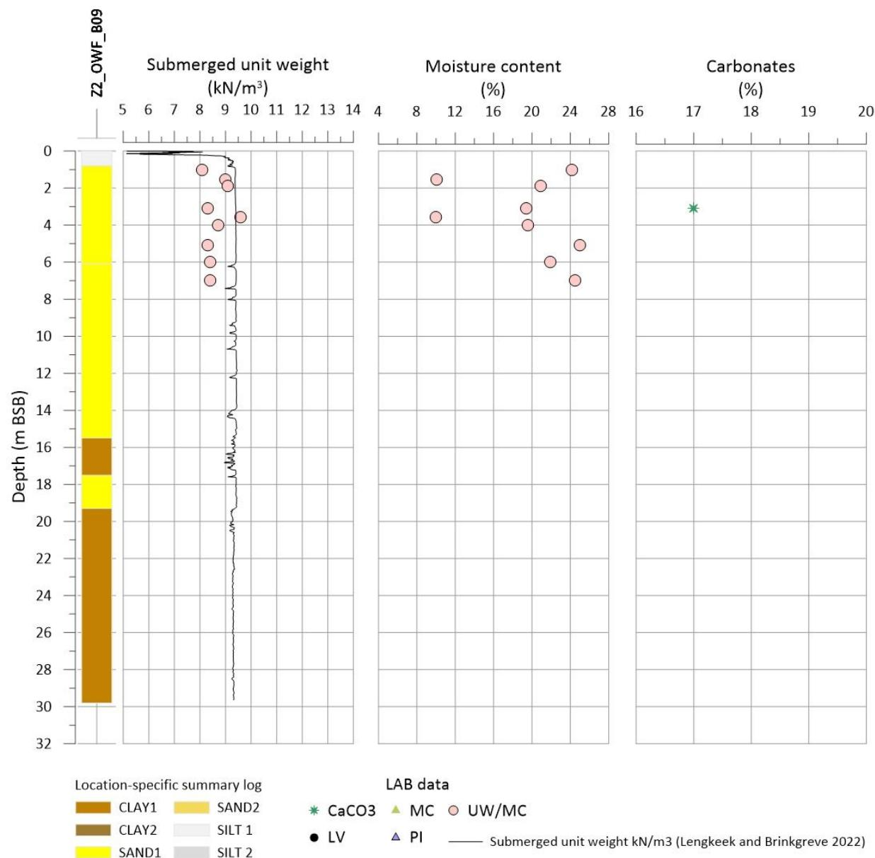
**Figure 11-19** Submerged unit weight, moisture content and Carbonate content for Z2\_OWF\_B09.
