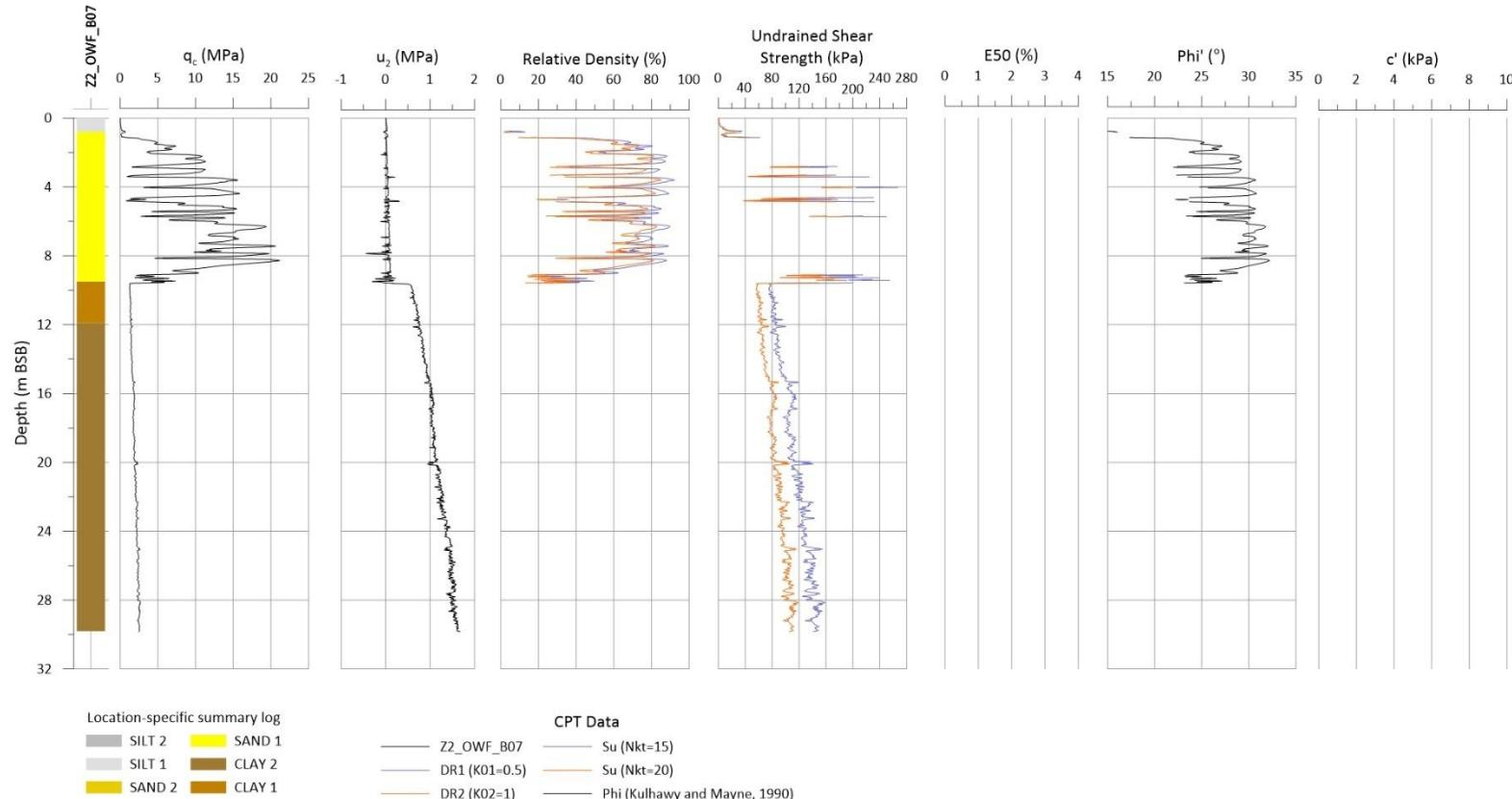
**Figure 11-15** qc, u<sub>2</sub>, relative density, Su, E50, Phi' and c' for Z2\_OWF\_B07.
