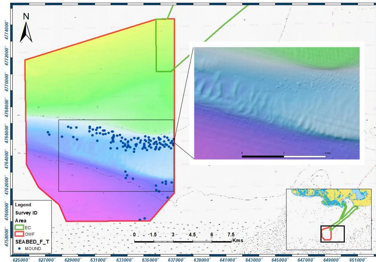
**Figure 7-6** Magnified view of seabed mounds in the center area of the OWF.
