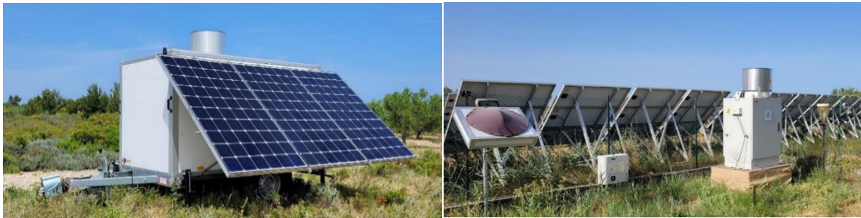
Equipment deployed for bird radar tracking on the coast. On the left, the mobile radar unit and on the right, the stationary radar installed at the Domaine de la Palissade (Camargue).
