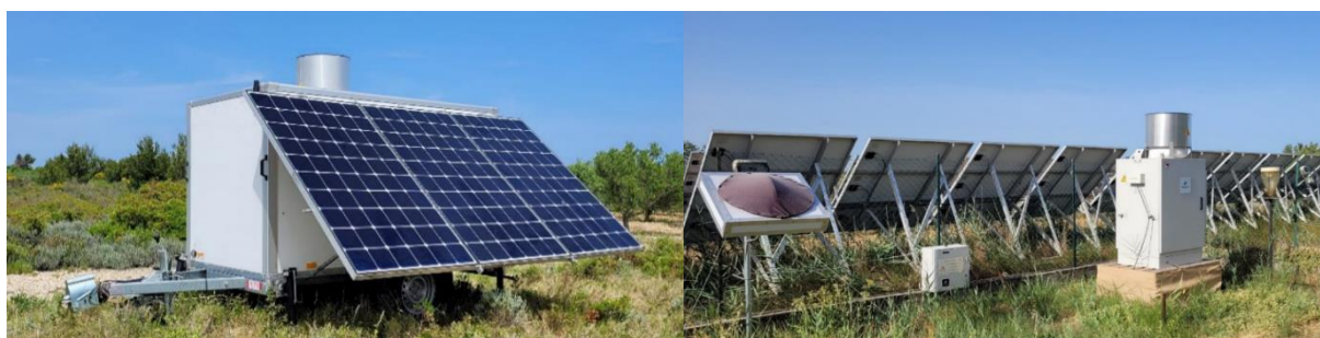
Figure 28 : Equipment deployed for bird radar tracking on the coast. On the left, the mobile radar unit and on the right, the stationary radar installed at the Domaine de la Palissade (Camargue).
