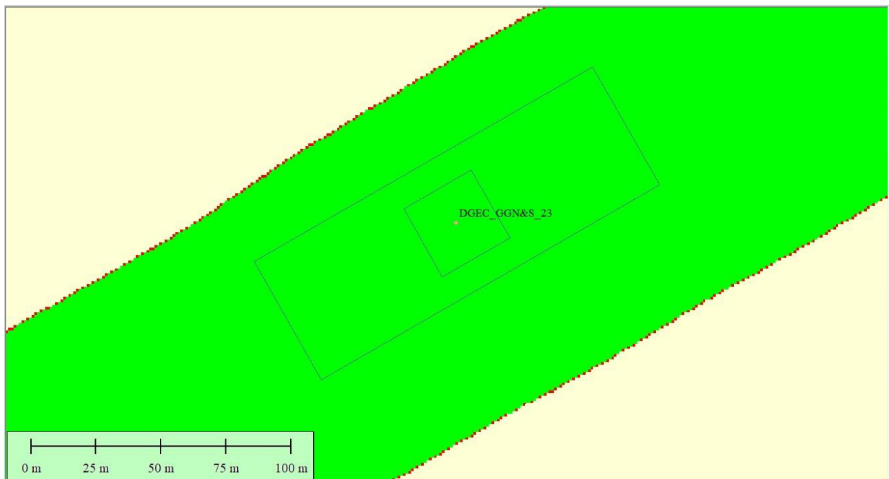
Figure 5-3: Survey box BOX_GI23 MBES data hit count 1 m per square (green means >30 hits per bin)
