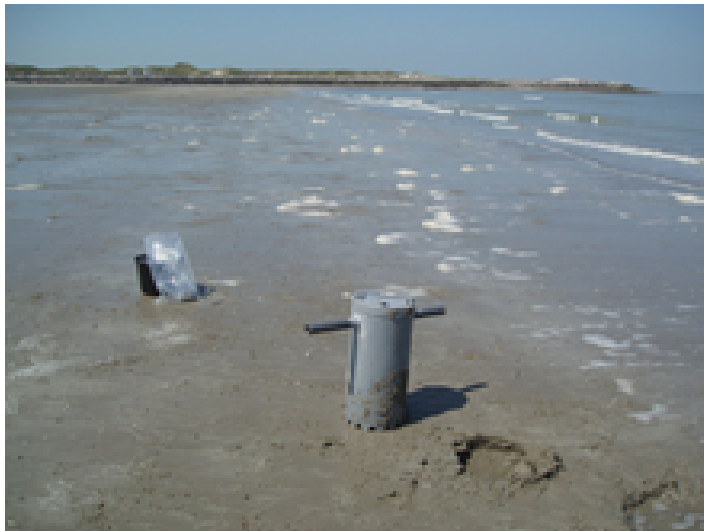
Figure 3 : Carottier à main (Cliché TBM)
