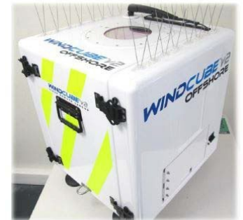
Figure 13 : Windcube V2 Offshore for floating platform (source : Leosphere)
